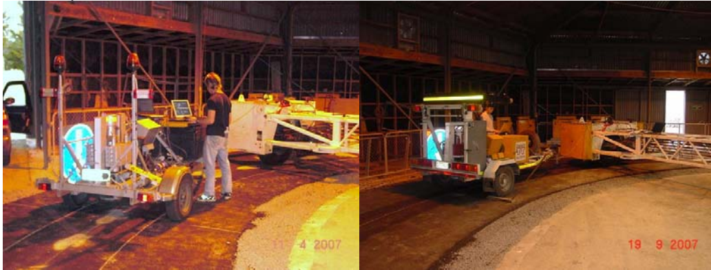
Figure 9 (a) FWD testing before trafficking (b) FWD testing after the application of 1 million load cycles
