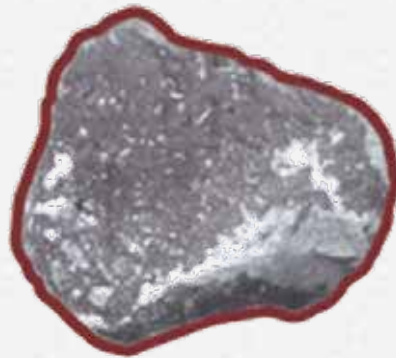
HARDER LIQUID TRANSFERRED FROM RAP PREVENTS STRIPPING
