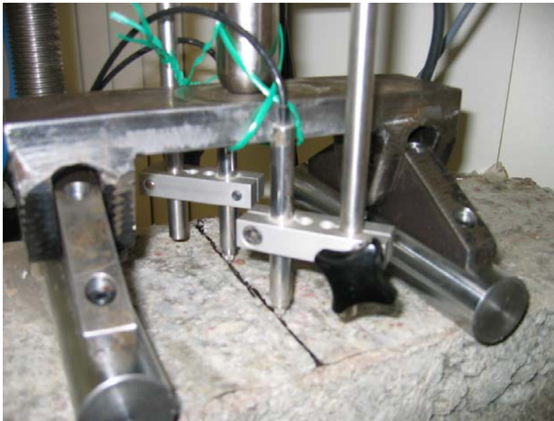
Figure 18 – Measuring deflection during the flexural beam test using LVDT's (Linear Variable Displacement Transducers)
