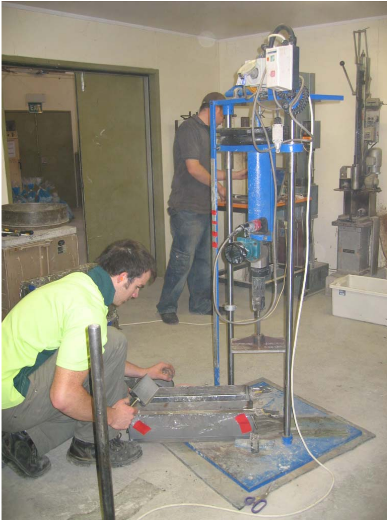
Figure 13 – Compaction frame with vibrating hammer and foot for beam manufacture.
