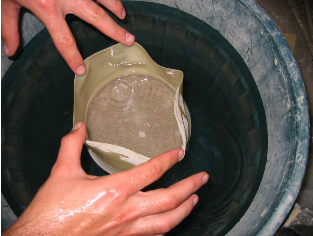
Figure 2 – Soaking sample for saturated undrained RLT test.
