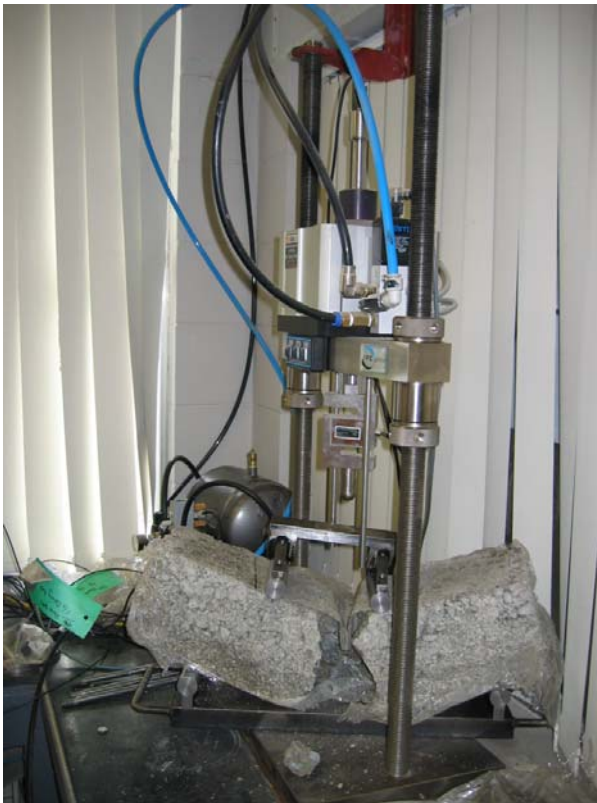
Figure 17 – Result after breakage or fatigue test.
