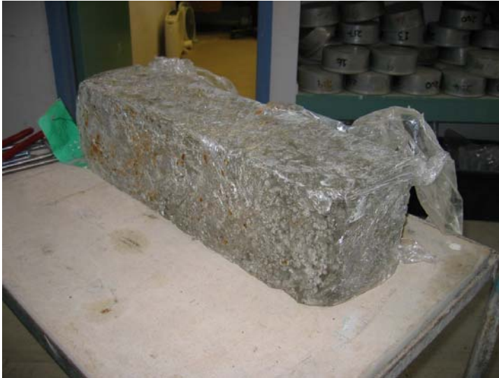
Figure 15 – Compacted and cured beam ready for testing.
