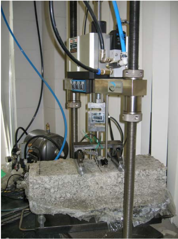
Figure 16 – Test setup for measuring flexural beam properties.
