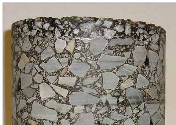
Figure 4: COMPACTASPHALT ® drill core – to demonstrate the intensive interlocking of the courses, a thin aluminium sheet was laid upon the binder prior to applying the upper-layer material.
