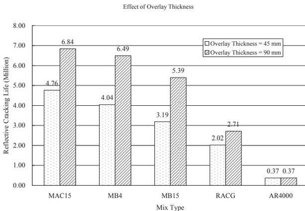
**Figure 20.** Effects of AC overlay thickness on reflective cracking life for different AC mixes.
