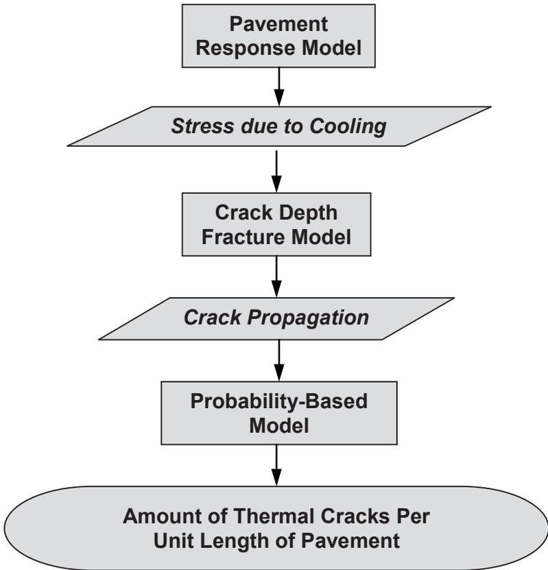
**Figure 1.** SHRP A-005 Thermal Cracking Model (Vinson *et al*, 1989)
