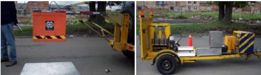
**Figure 10.** *GPR and FWD used on the survey*
