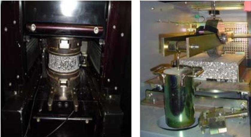
Figure 5. RSST-CH and Wheel tracking equipments
