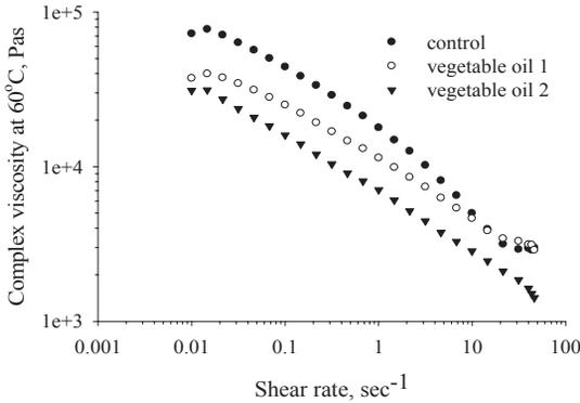
**Figure 2.** Viscosity decreasing effects of different treating methods at 0.1wt% oil concentration.
