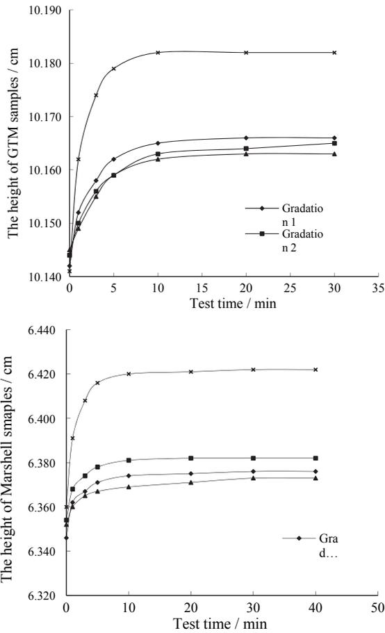
**Figure 3.** Linear expansion situation with different gradations and moulding modes over time
