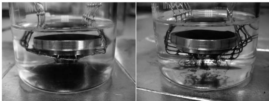
**Figure 2.** Binders solubility tests – CRM-0 (left) and CRM-20 (right) at  $t_{imm} = 1$  minute.
