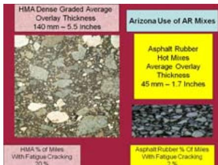
**Figure 10.** *ADOT AR Typical Thickness and Fatigued Cracking compared to Dense Graded HMA*
