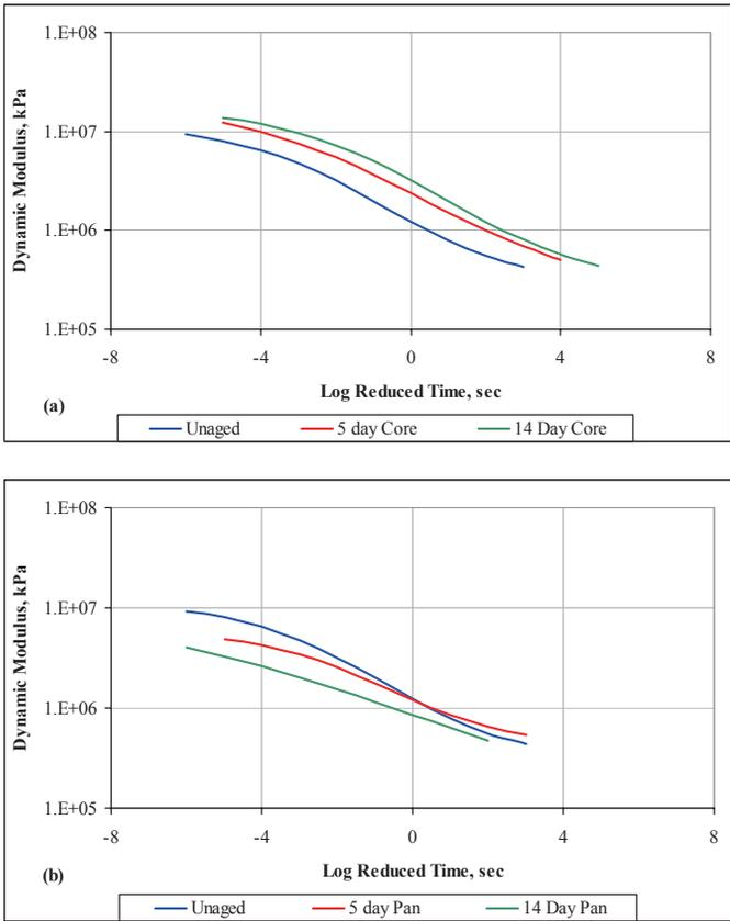
Figure 5. Dynamic Modulus Master Curves for ARFC Mixtures at (a) Core Aged (b) Pan Aged Conditions
