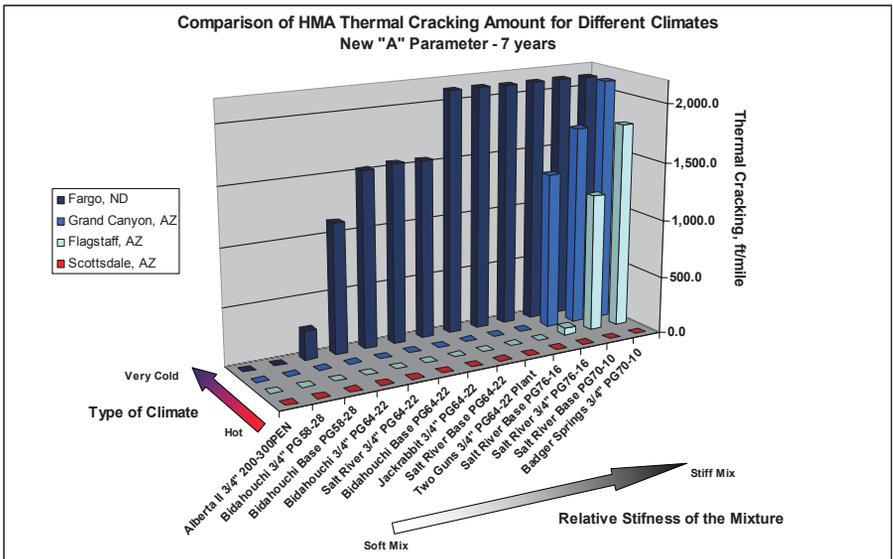
Figure 5. Predicted Thermal Cracking for Conventional Mixtures Using New Model
