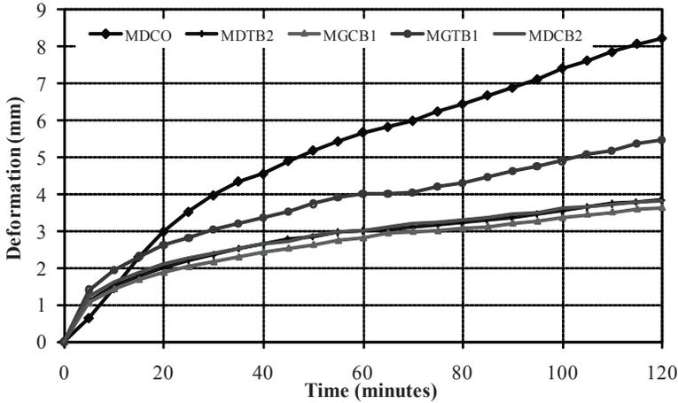
**Figure 7.** Evaluation of the deformation in the wheel tracking test
