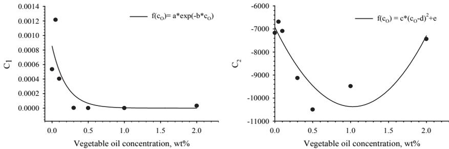
**Figure 4.** Viscosity-temperature correlation modelling by the Arrhenius equation
