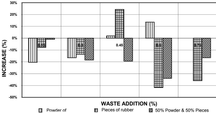
Figure 15. Effect of waste adding on rutting test.
