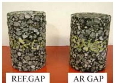
Figure 2. Malmo Highway E-06 Gap Graded Samples
