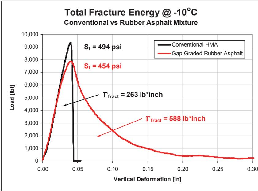
Figure 2. Total Fracture Energy Comparison for a Conventional and Asphalt Rubber Mixture
