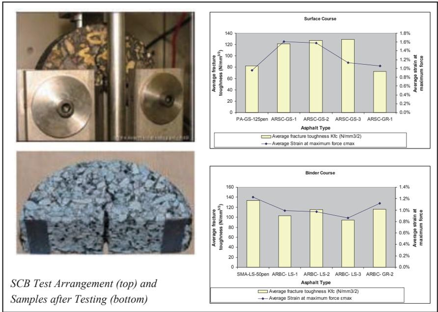
**Figure 8.** Crack Resistance at 0 °C
