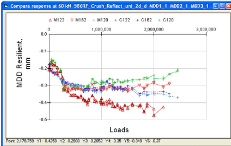
**Figure 10.** Measured (M, by MDD) and calculated (C) deflections, approximately on top of base
