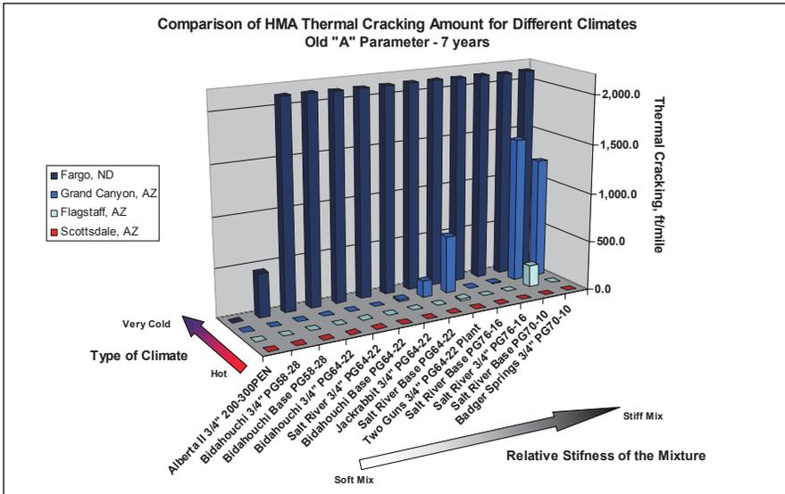
**Figure 4.** Predicted Thermal Cracking for Conventional Mixtures Using Old Model
