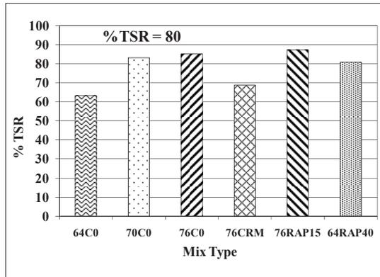
Figure 3. Modified Lottman Retained Tensile Strength
