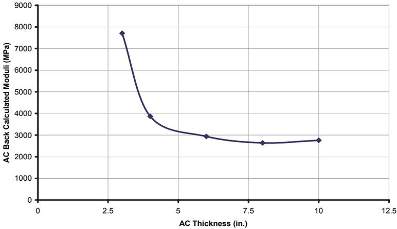
**Figure 15.** Effect of Thickness on the Back Calculated Moduli of the AC Layer
