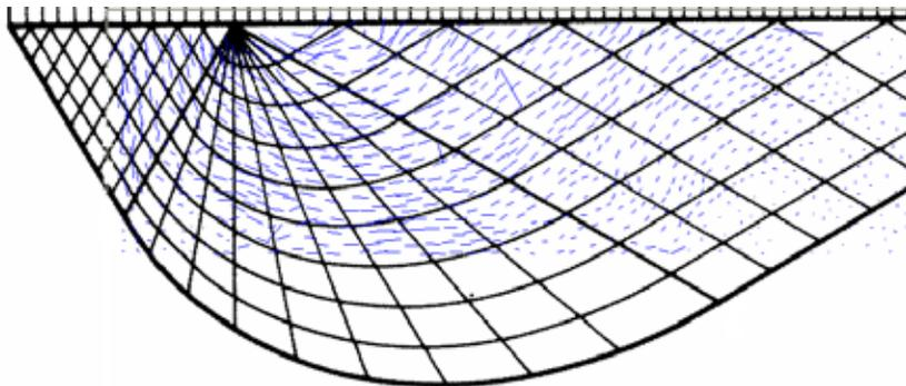
**Figure 3.** *Illustration of permanent deformation due to shearing*
