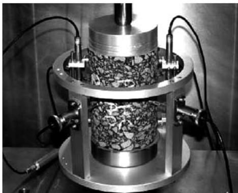
Figure 1. Typical E\* Dynamic Modulus Test Sample
