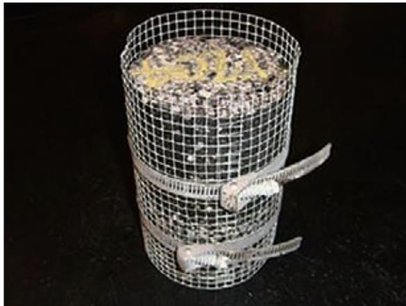
**Figure 2.** ARFC Sample Confined in Mesh Cage
