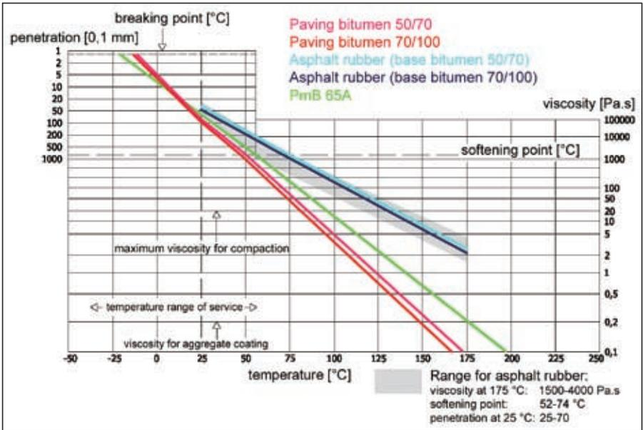
Figure 1. Temperature dependence characteristics of tested binders
