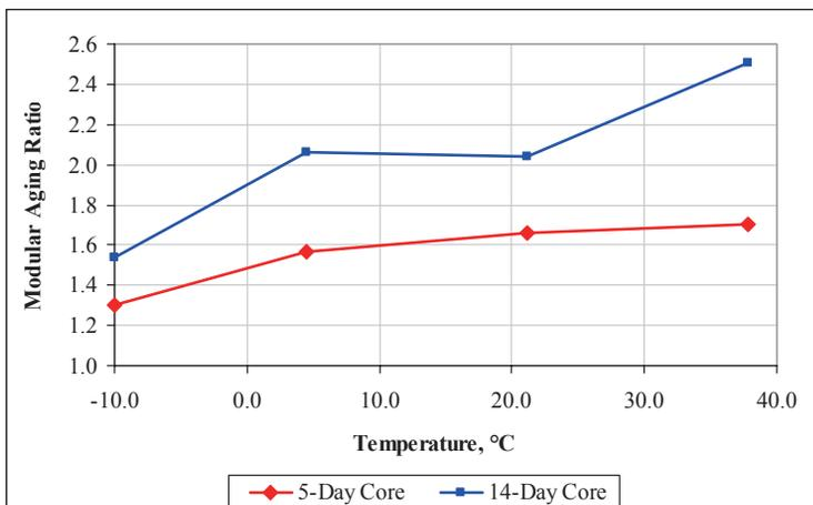
Figure 7. Modular Aging Ratio for ARFC, Core Aged
