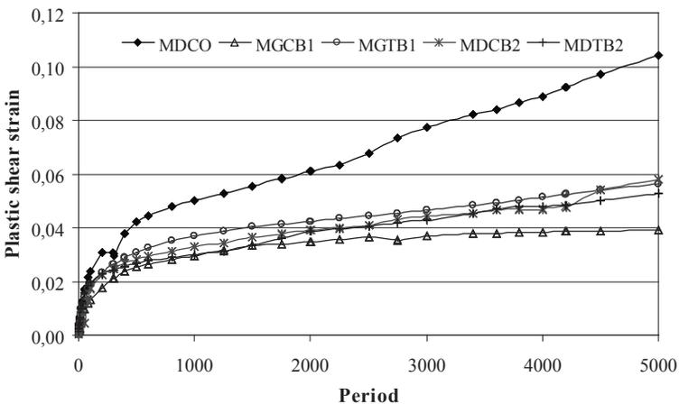
**Figure 6.** Development of the plastic shear strain in the RSST-CH tests
