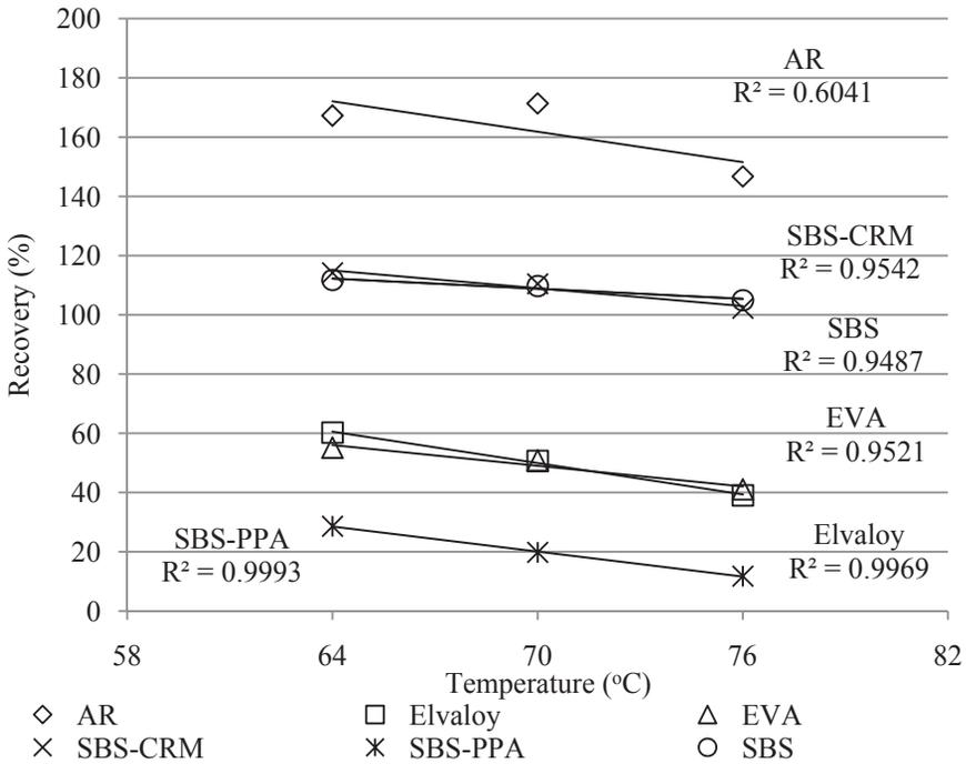
Figure 4. Percent recovery versus temperature
