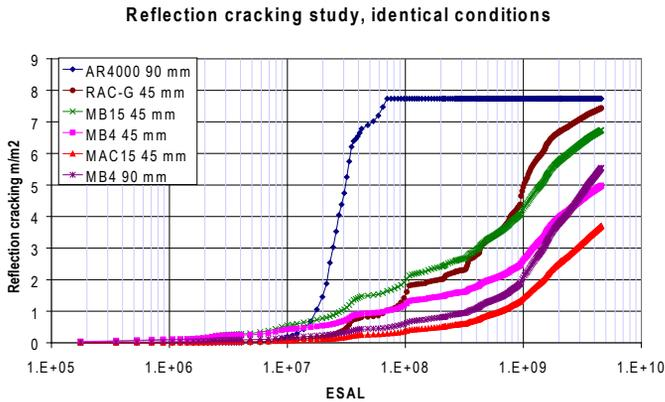
**Figure 17.** Reflection cracking study with identical underlying structure, loads and temperatures
