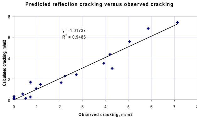
**Figure 15.** Predicted reflection cracking severity as a function of observed severity
