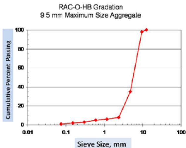
**Figure 2.** Typical aggregate gradation for RAC-O-HB (after Way 2007)
