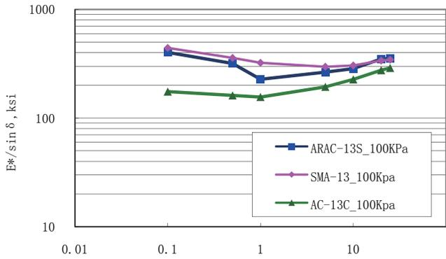
Figure 5.  $E^*/\sin\Phi$  (55°C, confined, 100kPa)
