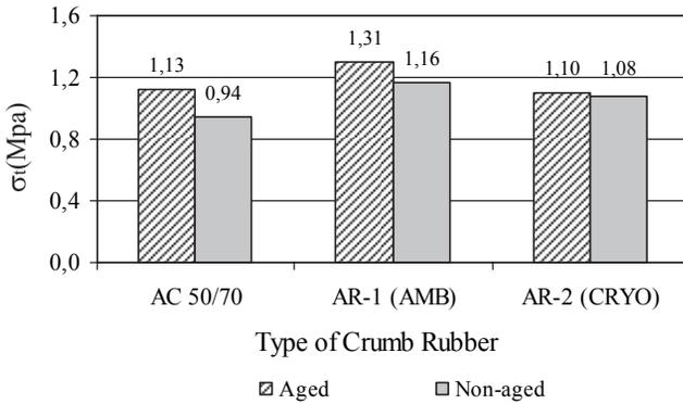
**Figure 6.** Indirect tensile strength of the dense graded asphalt hot mixes
