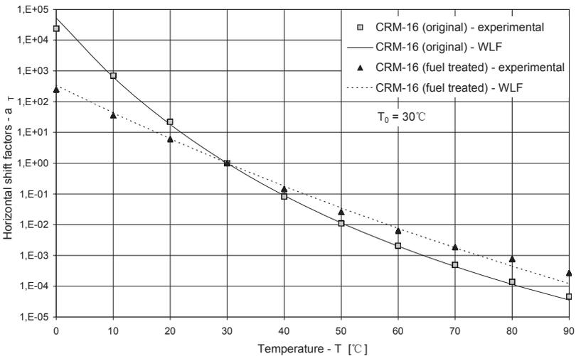
**Figure 6.** Shift factors for CRM-16 original and fuel treated (120 min. immersion).
