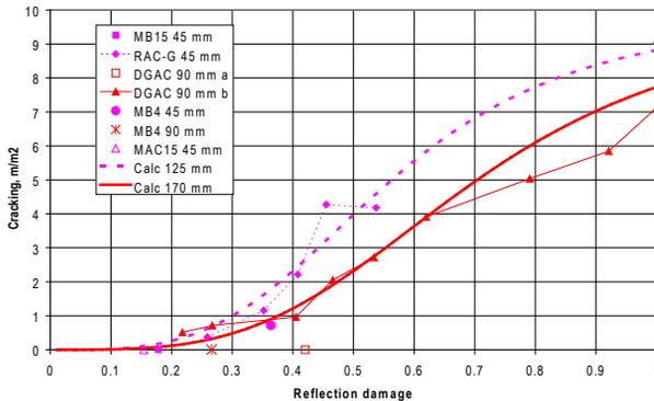
**Figure 14.** Surface cracking as a function of reflection damage
