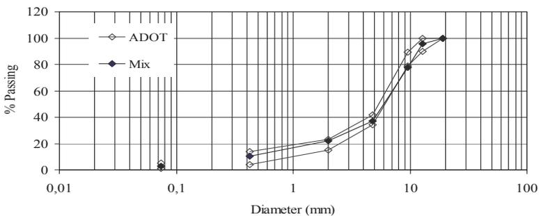
**Figure 1.** Grain size distribution curves for gap-graded mixes
