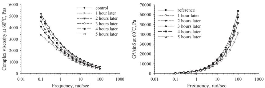
**Figure 7.** Hardening effect for AR binders (frequency vs. viscosity and  $G^*/\sin\delta$ ).
