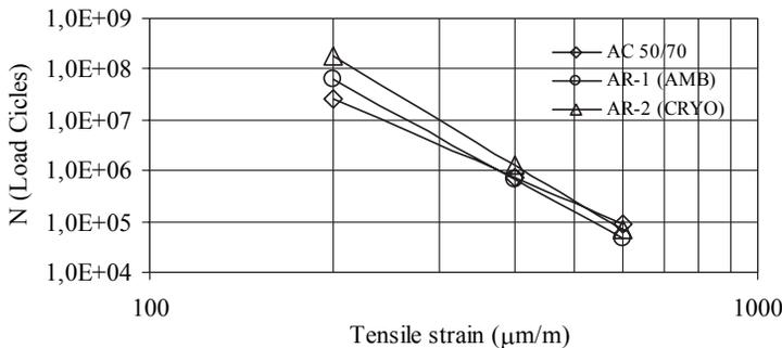
**Figure 9.** Fatigue life of dense graded asphalt hot mixes
