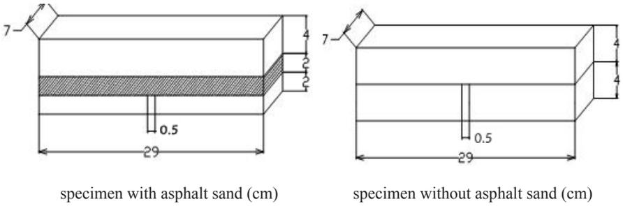
**Figure 1.** *Figuration of specimens*
