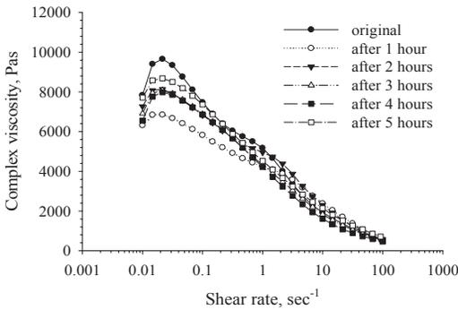
**Figure 8.** Hardening effect on viscosity curves (60°C) at 0.1% oil concentration.
