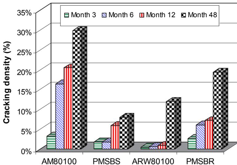
Figure 4. Cracking density in each section, after 4 year
