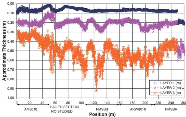
**Figure 11.** Asphalt pavement GPR profile
