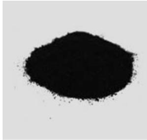
**Figure 1.** *Crumb rubber modifier (CRM) powder*
