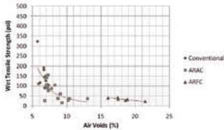
Figure 5. Wet Tensile Strength Versus Specimens Air Voids.
