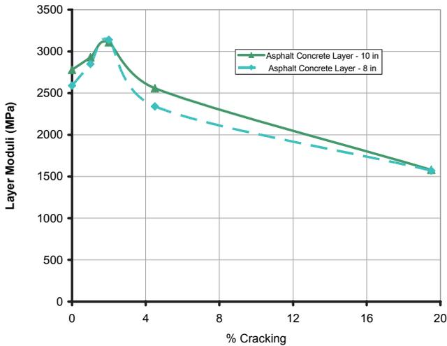
**Figure 17.** Variation of AC Layer Moduli with Cracking Level for 200 and 250 mm (8 and 10 in.) AC Thick Pavements
