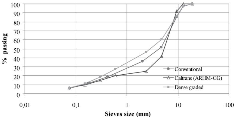
**Figure 2.** Aggregate gradation of studied mixtures
