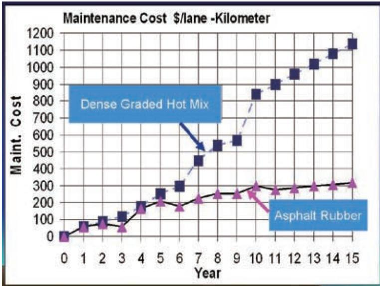
**Figure 15.** Pavement maintenance cost in \$/lane-Km versus years of service for HMA and asphalt-rubber pavements
