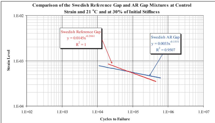
Figure 8. Comparison of Fatigue Relationships at 30% of Initial Stiffness
