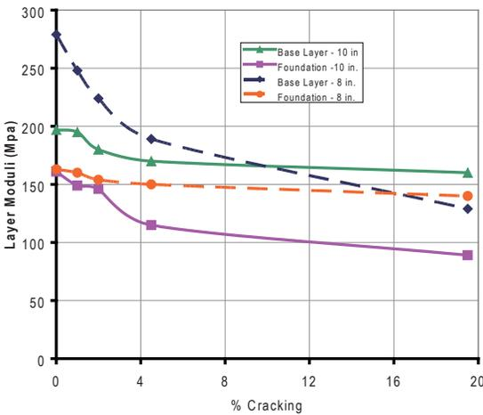
**Figure 16.** Variation of AB Base and Subgrade moduli of 200 and 250 mm (8 and 10 in.) AC thick pavements with percent cracking levels
