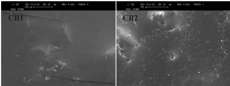
Figure 4. Microstructure of asphalts rubber binders CB1 and CB2
