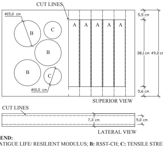
**Figure 5.** Specimens used in the laboratory tests
