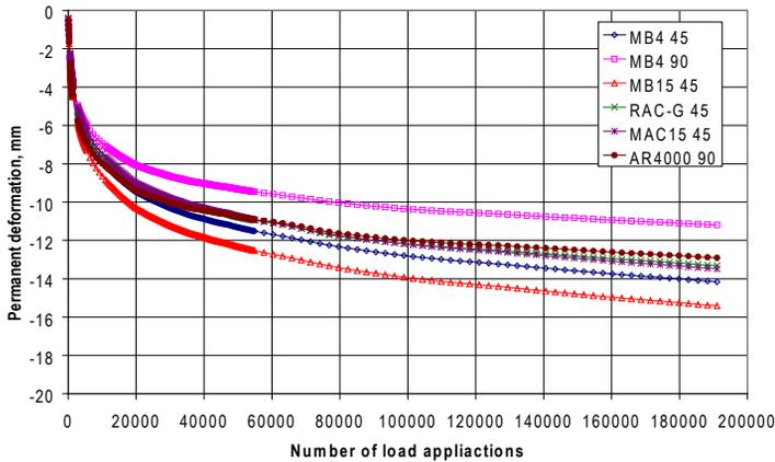
**Figure 16.** Result of rutting simulation with identical underlying structure, loads and temperatures.
