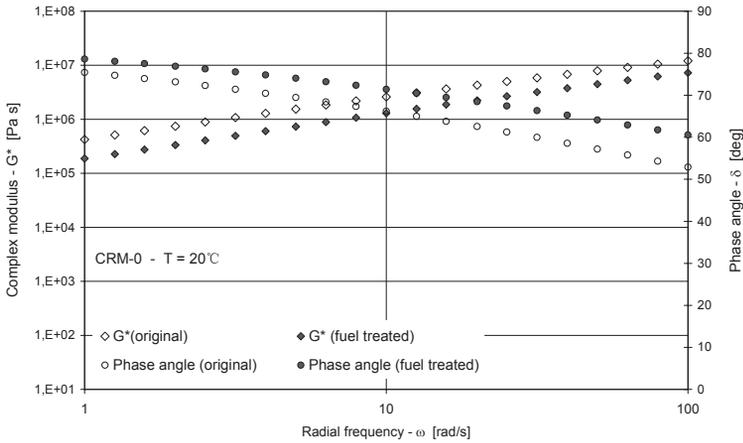
**Figure 3.**  $|G^*|$  and  $\delta$  at 20°C (CRM-0 original and fuel treated).
