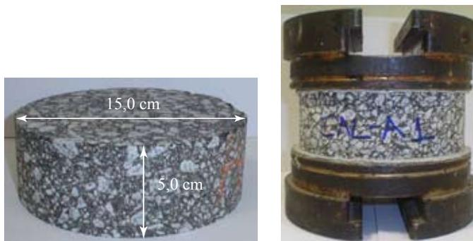
**Figure 3.** RSST-CH specimen dimensions and glued to caps
