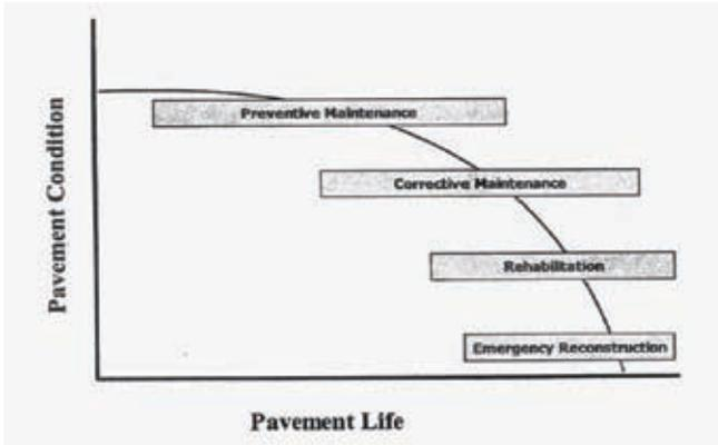
**Figure 1.** *Pavement Condition vs. Life and Type of Work Required*
