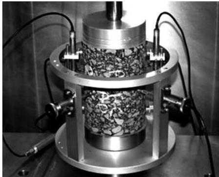
**Figure 5.** *Vertical and Radial LVDTs Set Up for an Unconfined Flow Number Test*
