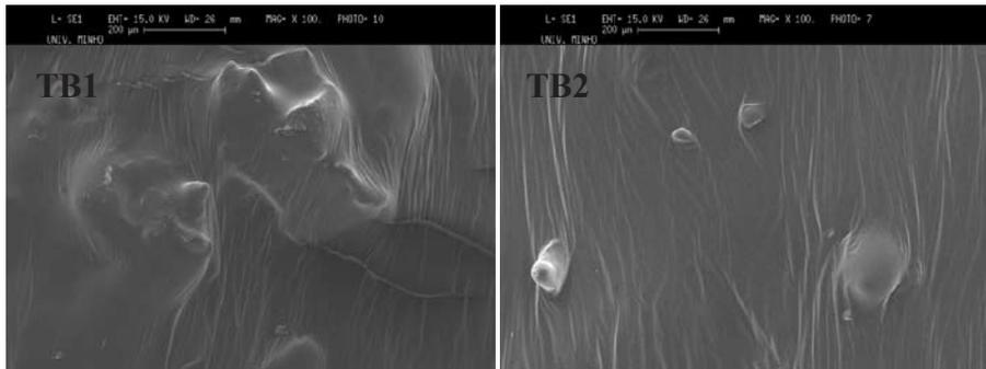
Figure 5. Microstructure of asphalts rubber binders TB1 and TB2
