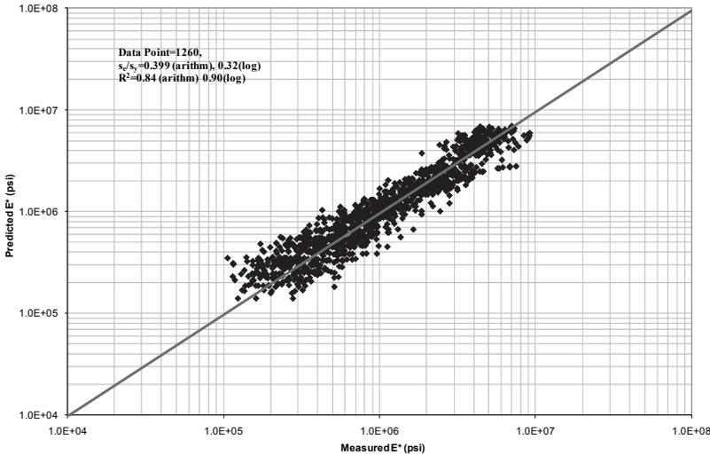
**Figure 4.** Dynamic Modulus measured versus predicted (Confined AR mixes)
