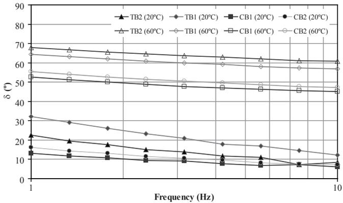
Figure 9. Asphalt rubber binder phase angles
