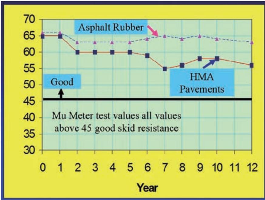
**Figure 16.** Pavement Mu Meter test values for skid resistance versus years of service for HMA and asphalt-rubber pavements
