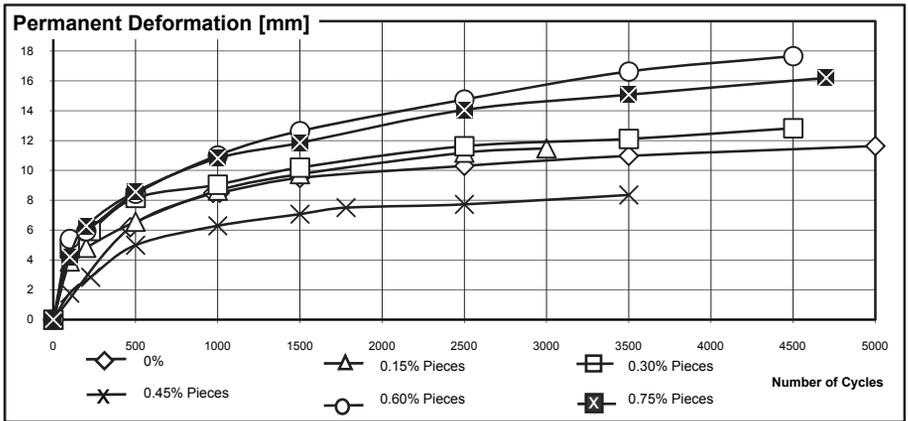
Figure 13. Increase of rutting versus number of cycles for pieces of rubber adding.
