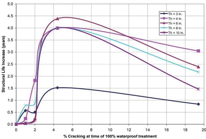
**Figure 14.** Structural Life Increase as a Function of cracking Level for Several Pavement Thicknesses (using 100% waterproof treatments)
