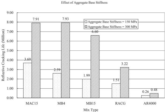
**Figure 21.** Effects of aggregate base stiffness on reflective cracking life for different AC mixes.
