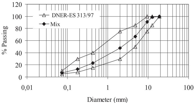
**Figure 4.** Grain size distribution curves for dense graded mixes
