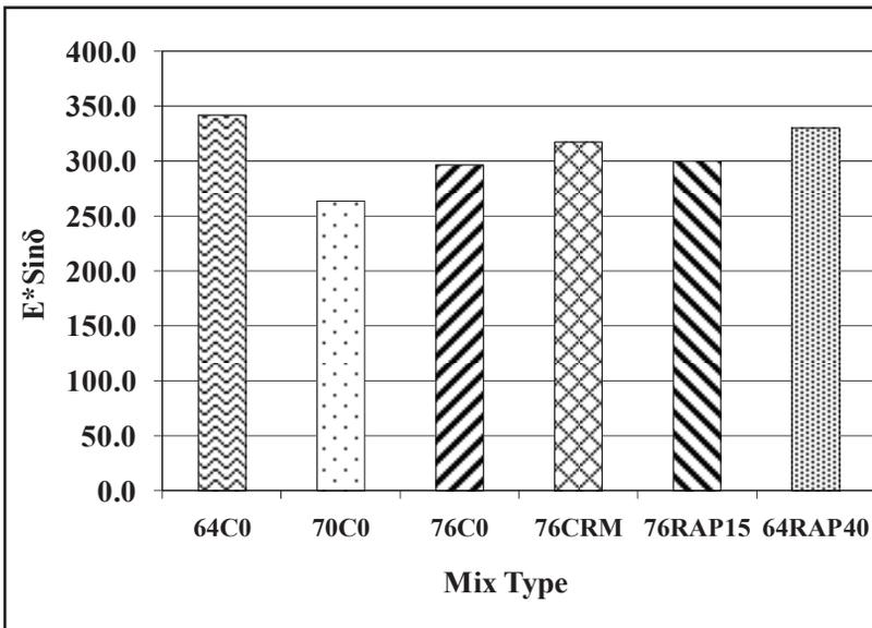
Figure 9. Fatigue factor,  $E^*(\text{Sin}\delta)$  @ 5Hz, 25.0 □
