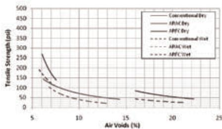
Figure 5. Tensile Strength Trends Versus Specimens Air Voids.
