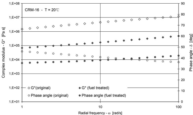
**Figure 4.**  $|G^*|$  and  $\delta$  at 20°C (CRM-16 original and fuel treated).
