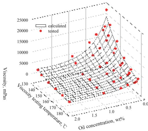
**Figure 5.** Modelling of viscosity affected by different vegetable oil content by using Eq. 2 optimized constant values ( $R^2=0.98$ )
