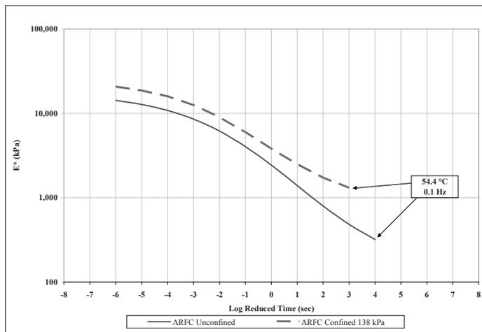
**Figure 3.** Dynamic Modulus Master Curves for ARFC Mixtures at Unconfined and Confined
