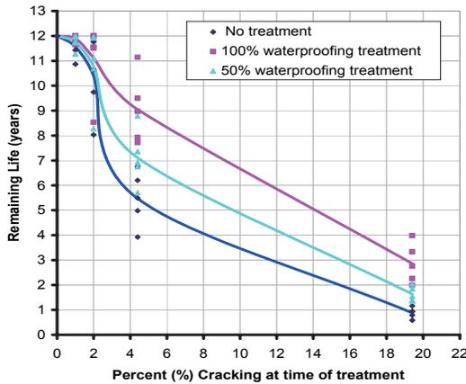
**Figure 12.** *Pavement Remaining Structural Life vs. Cracking Level (based on data at 1, 2, 4.5% and 18% cracking) (no best fit)*
