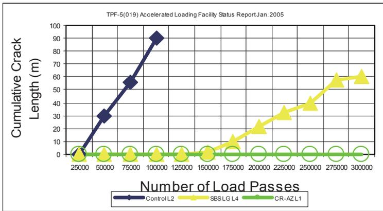
**Figure 9.** ALF-FHWA data relating number of passes and cracking level for three pavements with the same thickness (10 cm control- conventional, 10cm SBSLGL4- PMB binder and CR-AZL1- with 5 cm of asphalt rubber binder over 5 cm of conventional).
