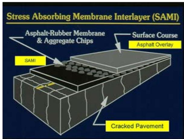
**Figure 6.** Asphalt-rubber Stress Absorbing Membrane Interlayer (SAMI)
