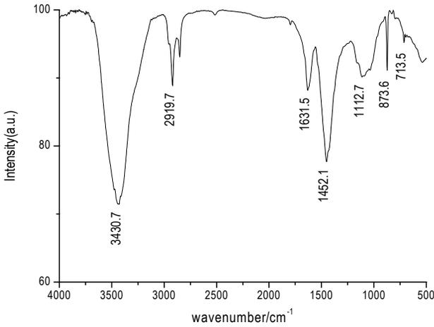
**Figure 1.** *Infrared absorption spectrum of waste rubber powder*
