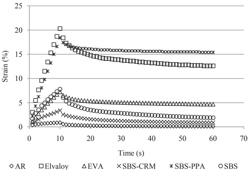
Figure 2. First cycle at 70°C and 100 Pa
