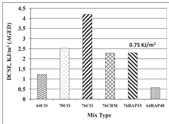
Figure 4. Dissipated Creep Strain Energy Test Results
