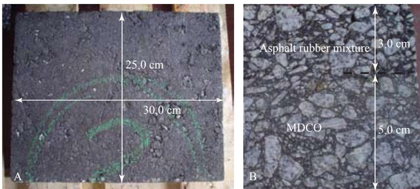
**Figure 4.** Wheel tracking slab (A: dimensions in plan view; in B, cross section view showing the configuration adopted for asphalt rubber mixtures in the test)
