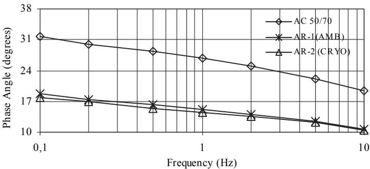
**Figure 8.** Phase angles of the dense graded asphalt hot mixes
