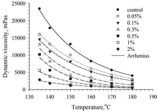
**Figure 3.** Viscosity-temperature correlation modelling by the Arrhenius equation
