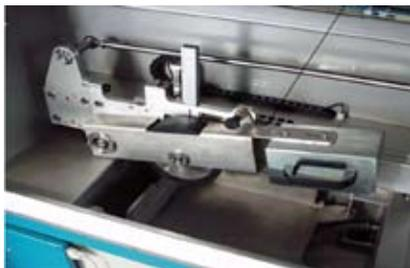
**Figure2.** Picture of the Hamburg wheel tracking test
