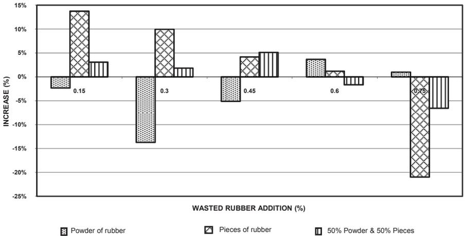
**Figure 9.** Increase of stability as function of waste addition for 75-blows of compaction level.
