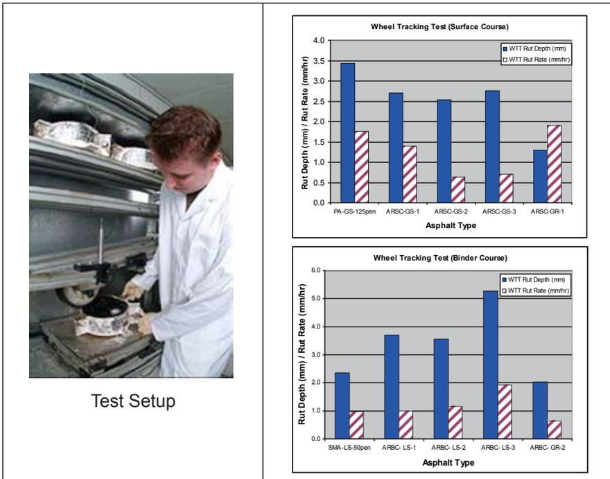
Figure 7. Wheel track testing at 60°C
