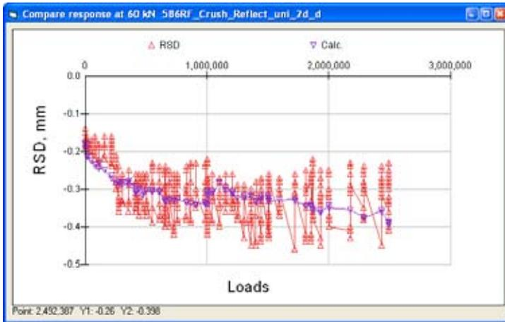
**Figure 8.** Measured (RSD) and calculated (Calc) surface deflection versus load applications
