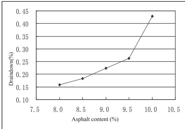
**Fig1.** Asphalt content VS draindown
