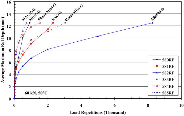
Figure 5. Rutting as a function of number of load applications
