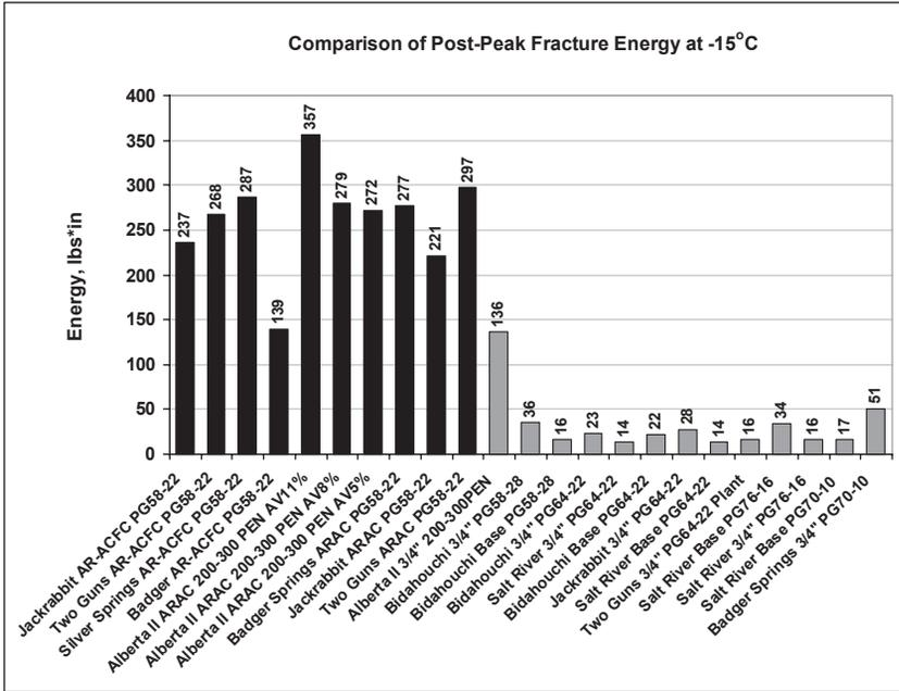
Figure 3. Differences in Post-Peak Fracture Energy Results at -15°C for Asphalt Rubber and Conventional HMA Mixtures (Black=Asphalt Rubber; Grey = Conventional).
