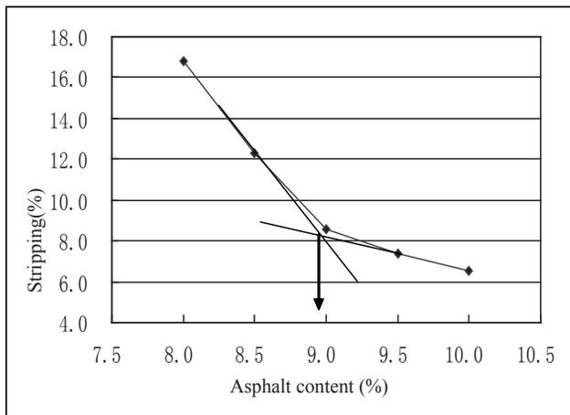
**Fig2.** Asphalt content VS stripping
