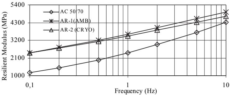
**Figure 7.** Resilient modulus of the dense graded asphalt hot mixes
