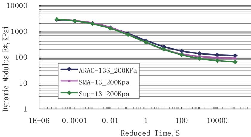
**Figure 3.** Dynamic Modulus Master Curve( 25°C, Confined, 200Kpa)
