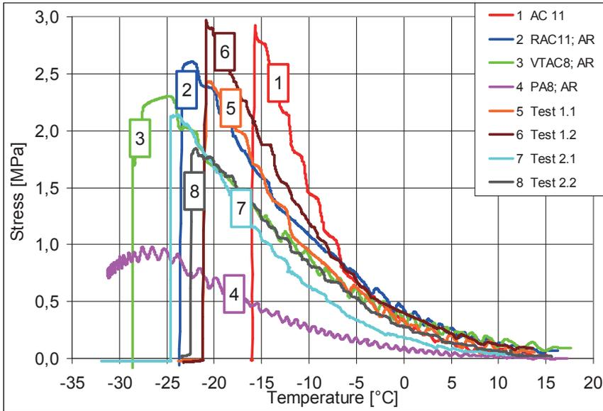
Figure 5. Dependence of thermal stress on temperature
