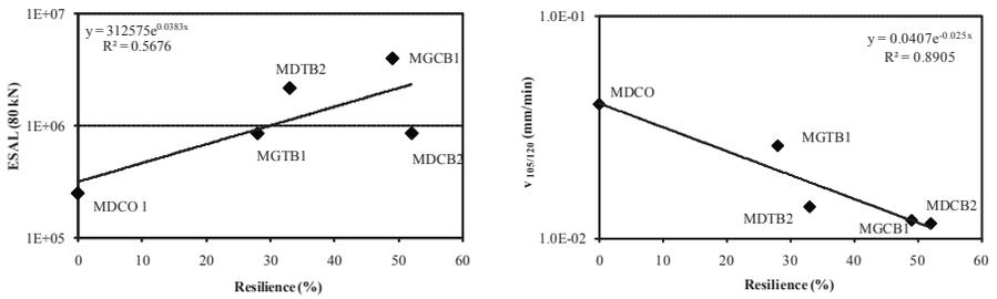
**Figure 13.** Relationship between resilience and ESAL (80 kN) and rate of deformation
