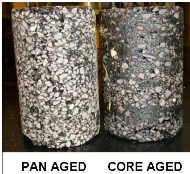
**Figure 3.** *Pan Aged versus Core Aged Specimen*
