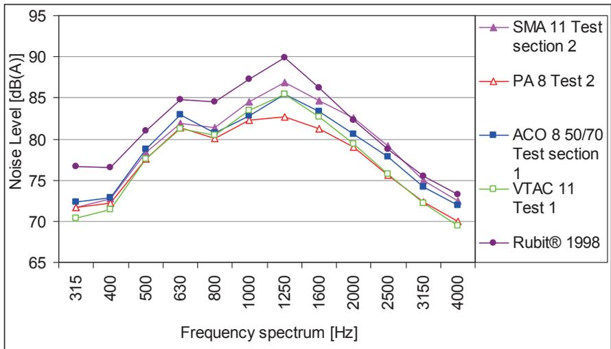
**Figure 8.** The evaluation of noise level by the form of third-octave characteristics of different wearing courses
