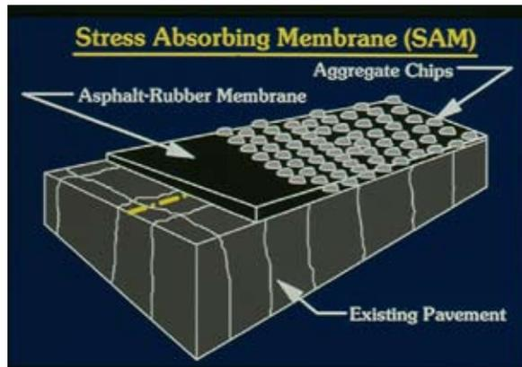
**Figure 5.** Asphalt-rubber Stress Absorbing Membrane (SAM)
