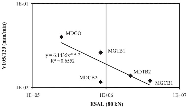
**Figure 10.** Comparison between RSST-CH and wheel tracking tests
