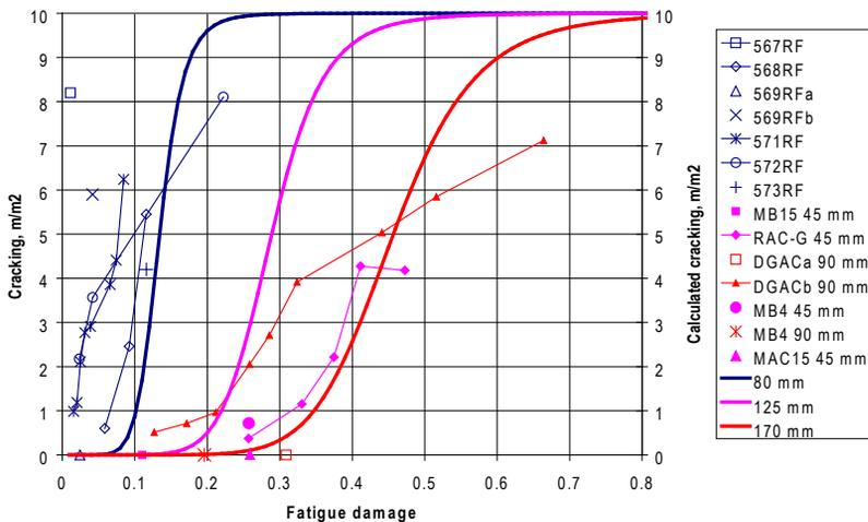
**Figure 13. Surface cracking as a function of fatigue damage**
