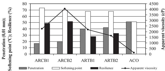
**Figure 1.** Characterization tests of the asphalts
