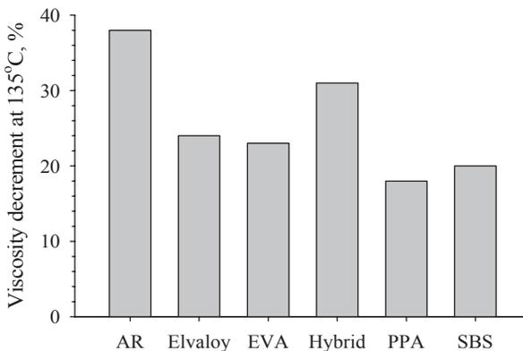
**Figure 6.** *Softening effect of vegetable oil at concentration of 0.1% (135°C).*
