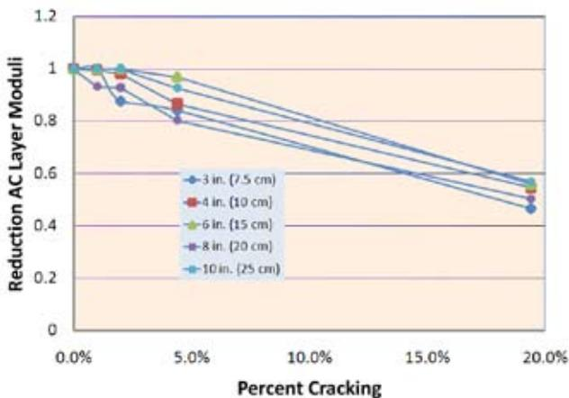
Figure 7. Reduction of AC Layer Moduli versus Percent Cracking
