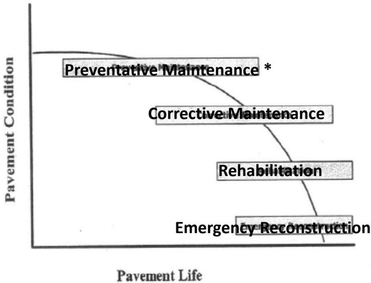
**Figure 1.** *Pavement Condition vs. Life and Type of Work Required*
