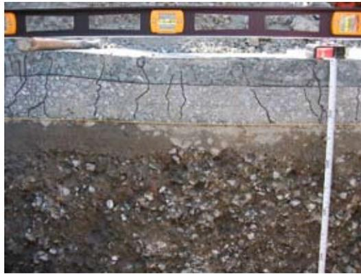
**Figure 7.** *Fatigue section forensic (cracks are highlighted with marker pen)*
