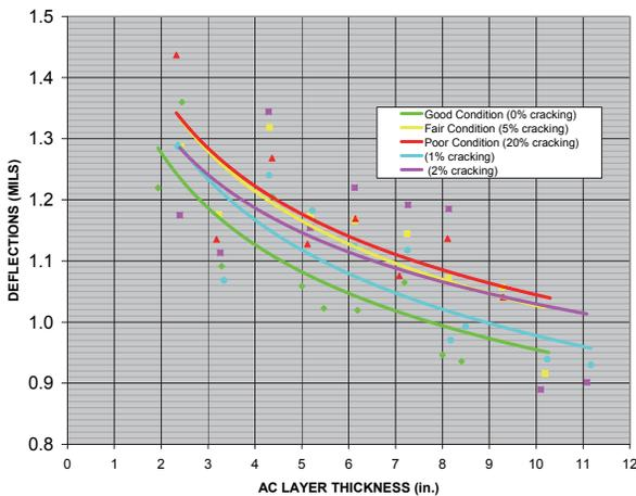
**Figure 13.** *FWD Geophone Number 7 (DF7) Deflection Related to the AC Layer Thickness and Level of Percent Cracking*
