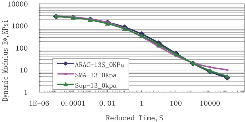
**Figure 1.** Dynamic Modulus Master Curve( 25°C, Unconfined )
