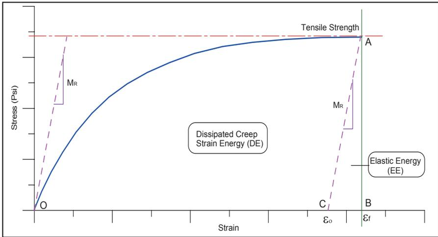
**Figure 1.** Dissipated Creep Strain Energy Determination
