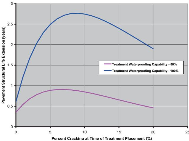
**Figure 11.** Structural Life Extension vs. Percent Cracking at Time of Treatment (based on data at 1, 2, 4.5 and 18.5%)
