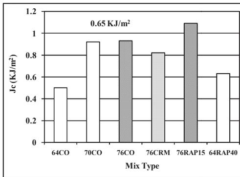
Figure 5. Semi-Circular Bend Test Results
