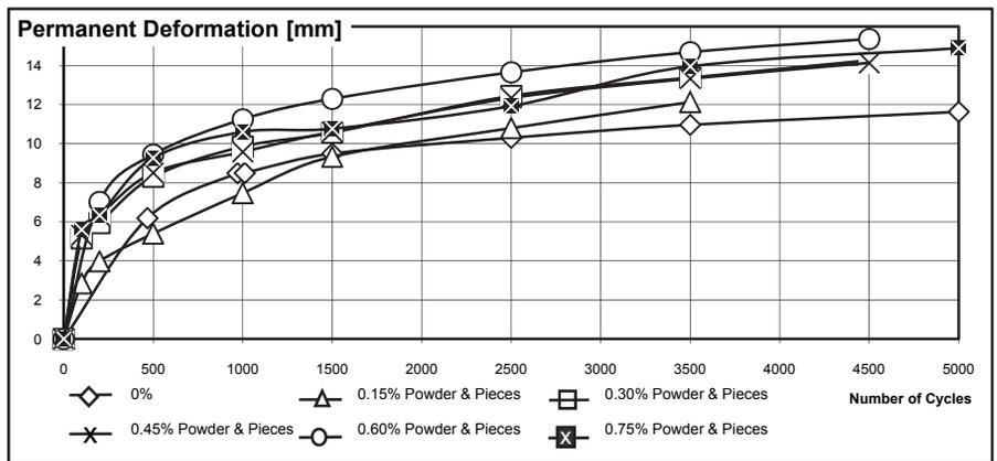
Figure 14. Increase of rutting versus number of cycles for combination of powder and pieces of rubber.
