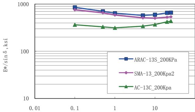
Figure 6.  $E^*/\sin\Phi$  (55°C, confined, 200kPa)
