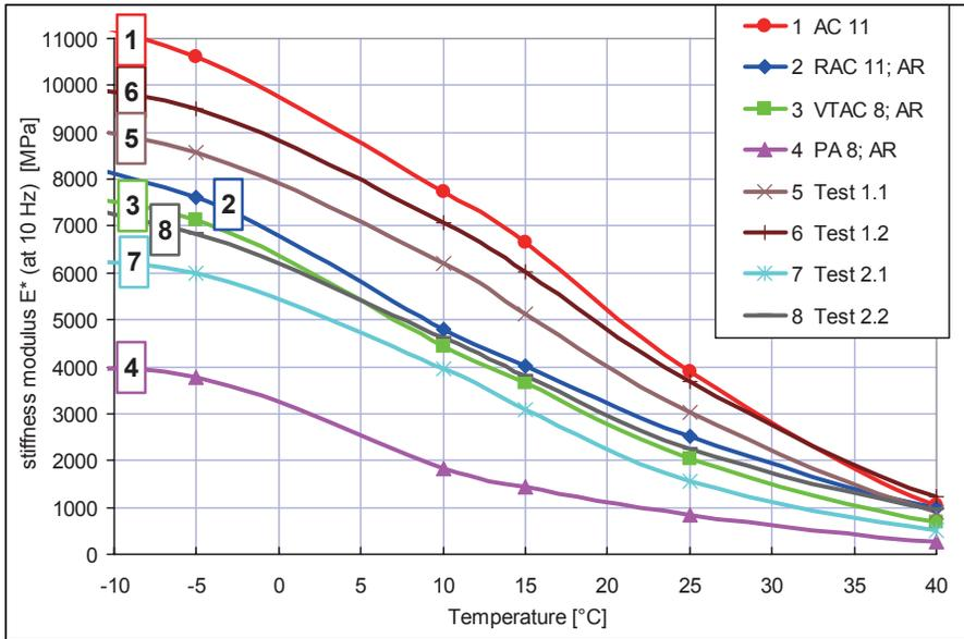
Figure 3. The dependence of stiffness on temperature at 10 Hz
