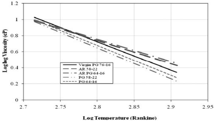
**Figure 1.** Viscosity-Temperature Susceptibility Comparison of Conventional and Crumb Rubber Modified Binders.
