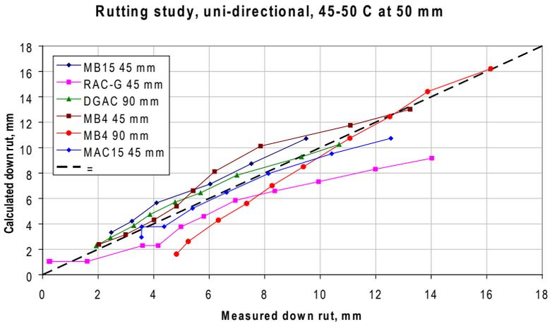
**Figure 11.** Measured and calculated down rut during rutting study
