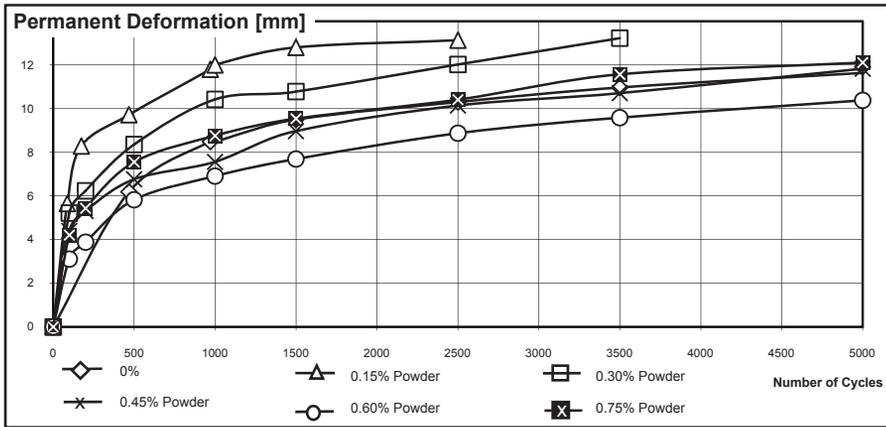
Figure 12. Increase of rutting versus number of cycles for powder of rubber adding.
