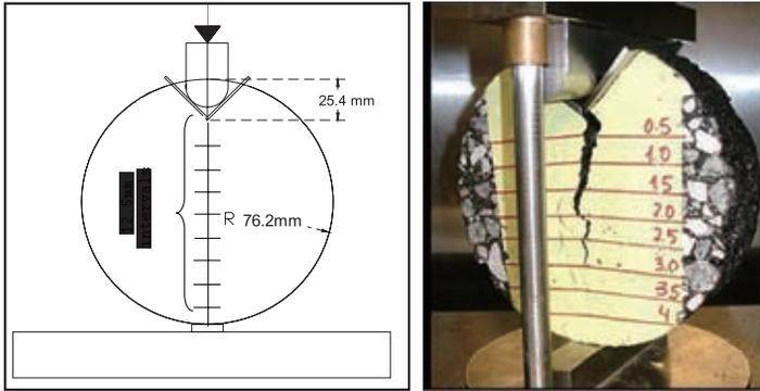
Figure 9. Typical  $C^*$  Test Setup
