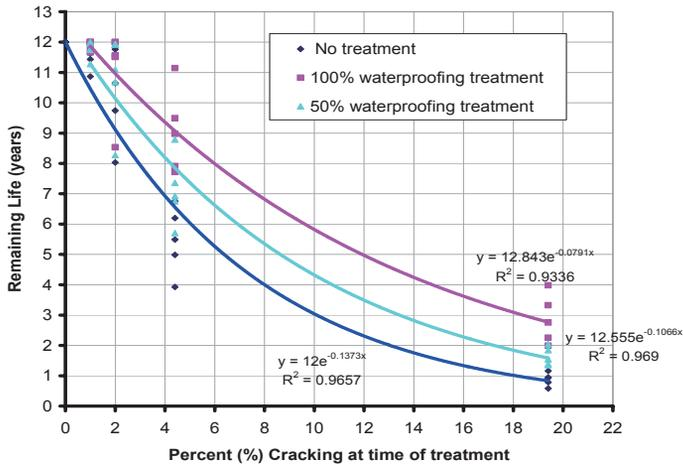
**Figure 10.** Pavement Remaining Structural Life vs. Cracking Level (based on data at 1, 2, 4.5 and 18% cracking)
