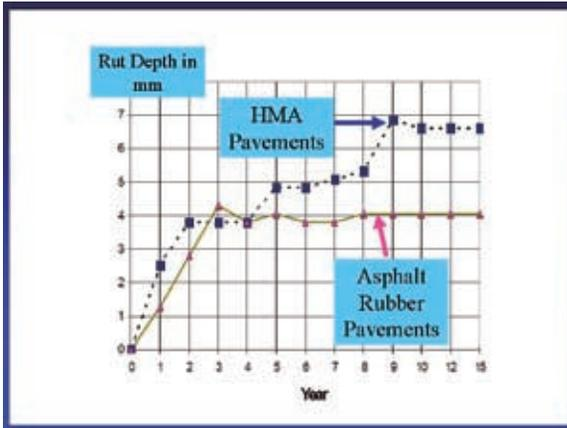
Figure 13. Rut depth in mm versus years of service for HMA and asphalt-rubber pavements
