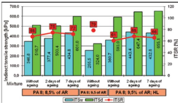
**Figure 2.** The results of indirect tensile strengths of Porous Rubber-Asphalt (PA 8) with different binder content, hydrated lime addition and ageing
