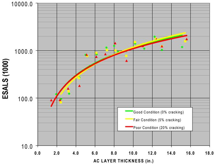
**Figure 5.** AC Pavement Layer Thickness versus ESAL's of Traffic Loading
