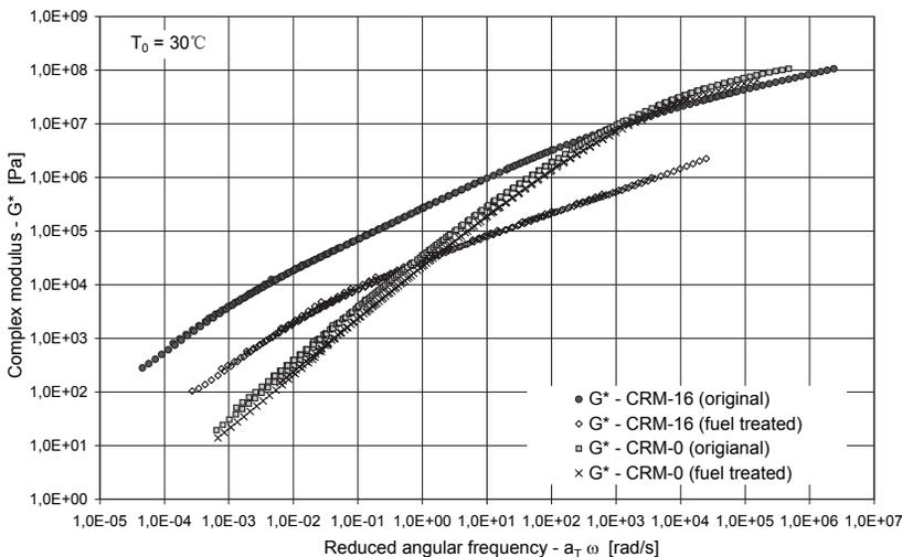
Figure 5.  $G^*$  master curve for CRM-0 and CRM-16 original and fuel treated (120 min. immersion).
