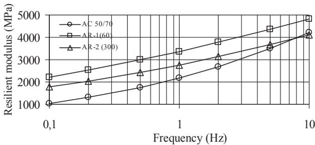
**Figure 3.** Resilient modulus of the gap-graded asphalt hot mixes
