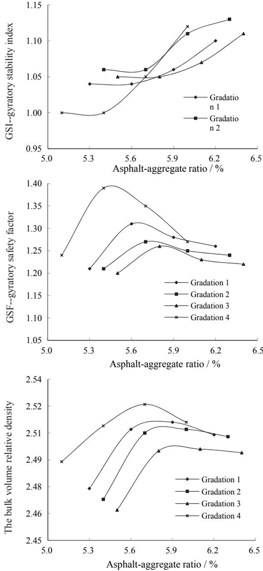
**Figure 2.** Changing regularity of the mechanical parameters and density of the GTM samples with the asphalt-aggregate ratios
