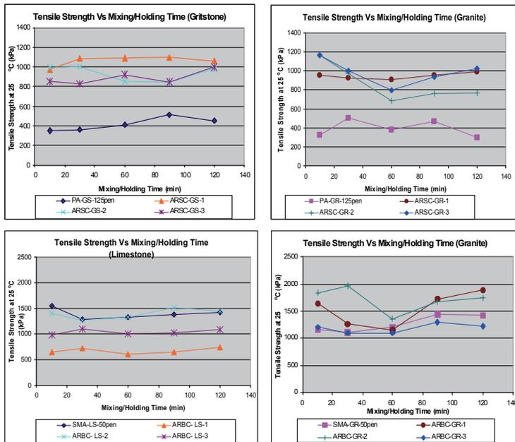
Figure 4. Tensile Strength Assessment – Results at 25°C
