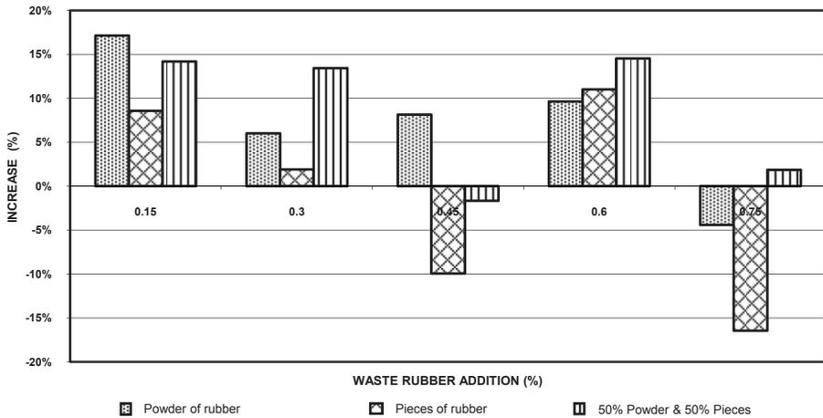
Figure 8. Increase of stability as function of waste addition for 50-blows of compaction level.
