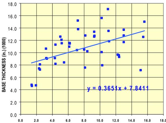
Figure 6. AC Pavement Layer Thickness versus Aggregate Base Layer Thickness
