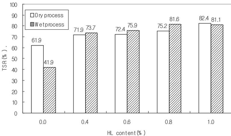
**Figure 3.** Comparison of TSR by HL contents and dry and wet process.
