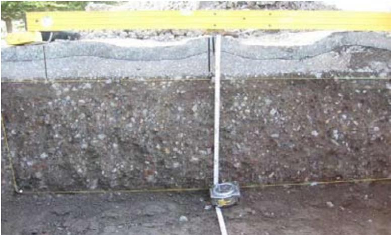
Figure 6. Rutting in the underlying DGAC on the 45-mm MB4-G Section
