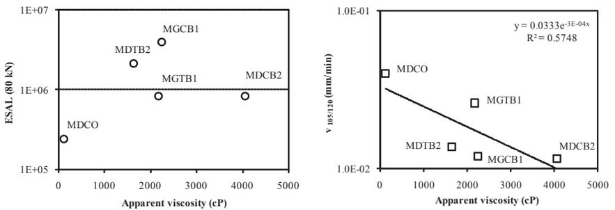
**Figure 14.** Relationship between apparent viscosity and ESAL (80 kN) and rate of deformation
