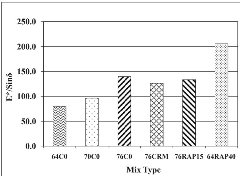
**Figure 8.** Rutting factor,  $E^*/\text{Sin}\delta$  @ 5Hz, 54.4 °C
