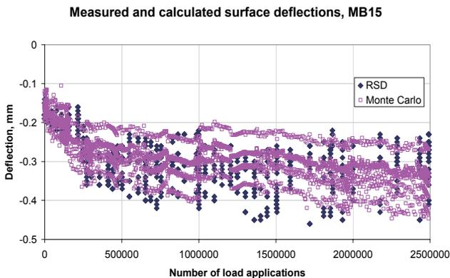
**Figure 9.** Monte Carlo simulation of the MB15 section
