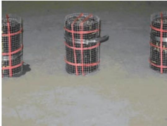
**Figure 3.** *Sample Wrapped with Thin Steel Wire Mesh*
