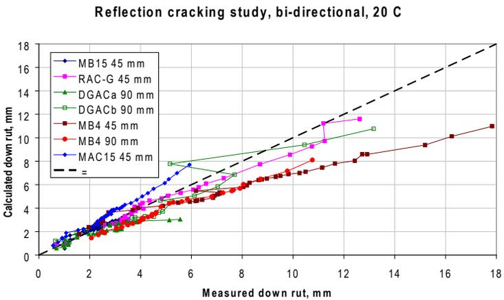
**Figure 12.** Measured and calculated down rut during reflection cracking study
