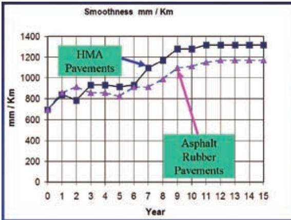
Figure 14. Pavement smoothness in mm/km versus years of service for HMA and asphalt-rubber pavements
