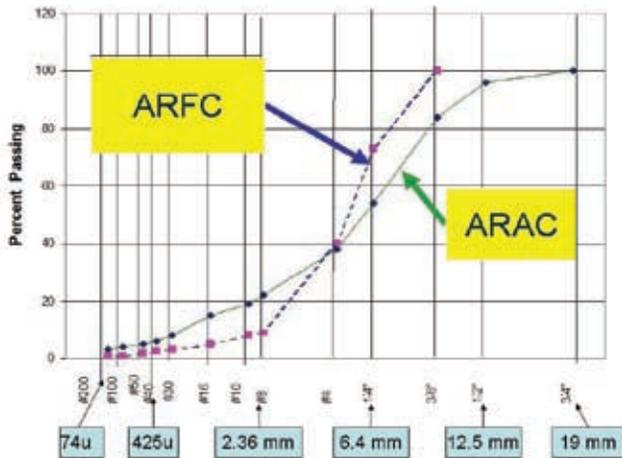
**Figure 9.** ADOT ARAC (Gap-Graded) & ARFC (Open Graded) Gradation Chart -Sieve Sizes to 0.45 Power
