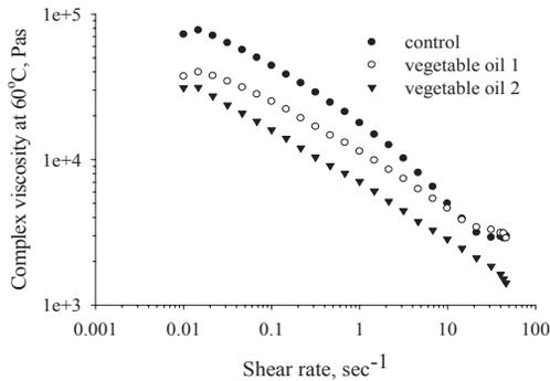
**Figure 1.** Viscosity decreasing effects of different vegetable oils at 0.1wt% concentration.
