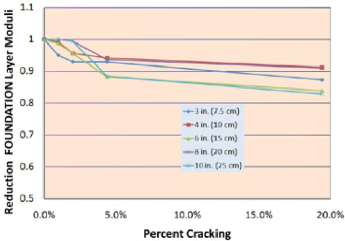
Figure 9. Reduction of Base Layer Moduli versus Percent Cracking
