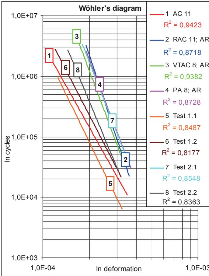
Figure 4. Fatigue properties of tested mixtures, temperature 10 °C, frequency 25 Hz
