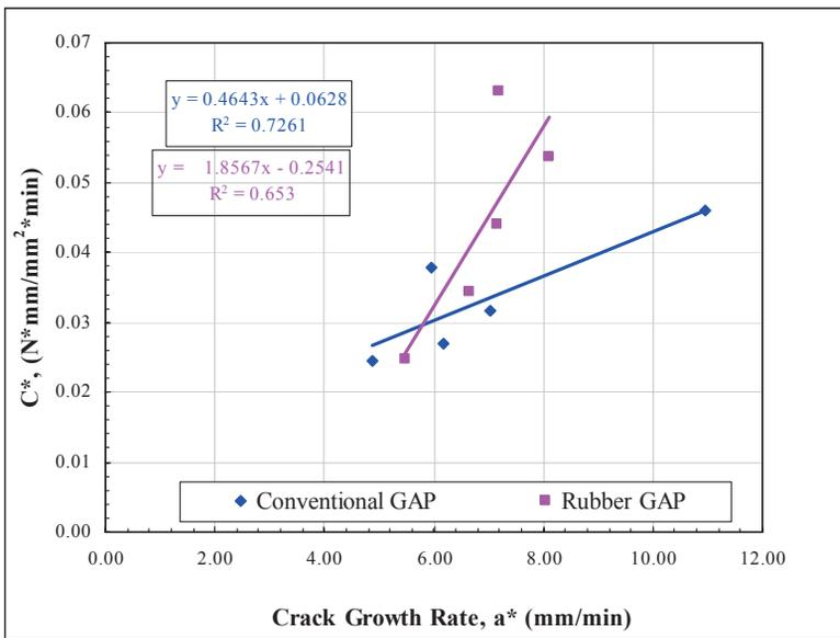
Figure 15. Crack Growth Rate versus  $C^*$  Values For Reference and Rubber Gap Mixes
