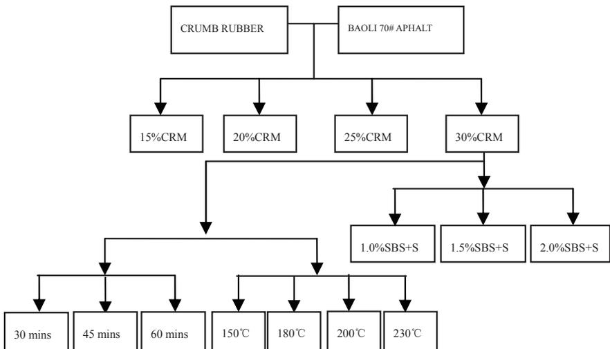
**Figure 1.** Flow chart of experimental design procedures
