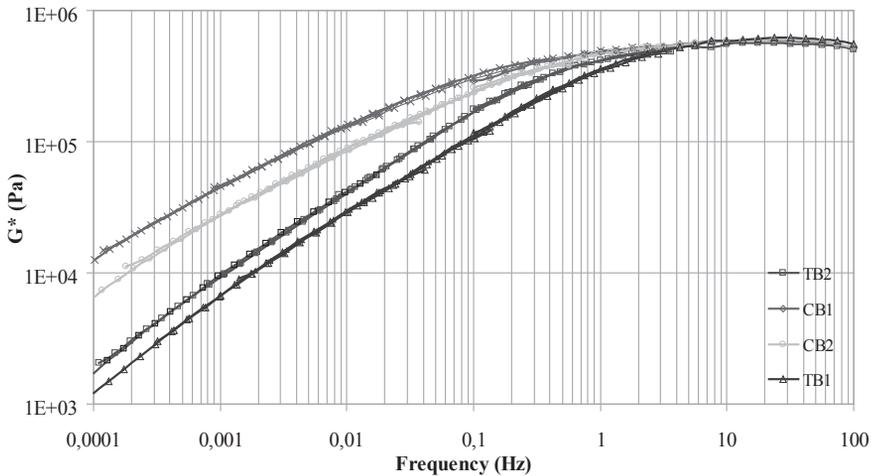
Figure 10. Master curves of the asphalt rubber binders
