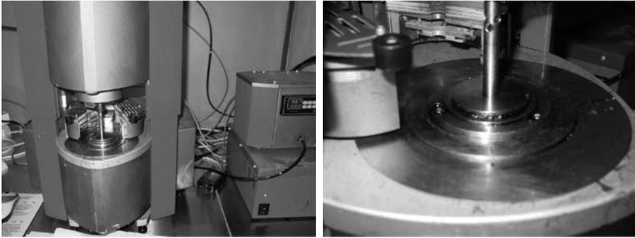
Figure 6. Rheometer and parallel plates
