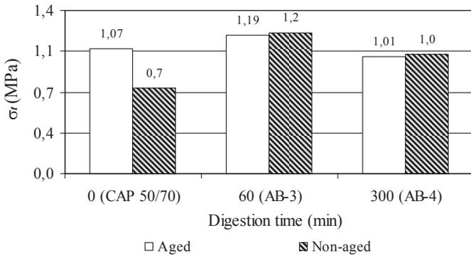
Figure 2. Indirect tensile strength of the gap-graded asphalt hot mixes
