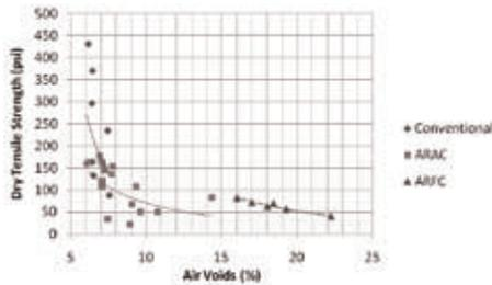
Figure 4. Dry Tensile Strength Versus Specimens Air Voids.
