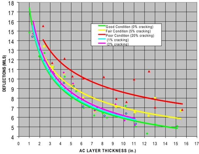
**Figure 4.** FWD Sensor Number 1 Deflection versus AC Pavement Layer Thickness
