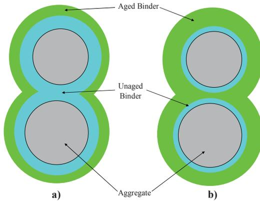
Figure 6. Schematic of Binder Coating on Aggregates at (a) Core (b) Pan Aged Conditions
