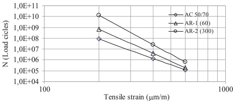
**Figure 5.** Fatigue life of gap-graded asphalt hot mixes
