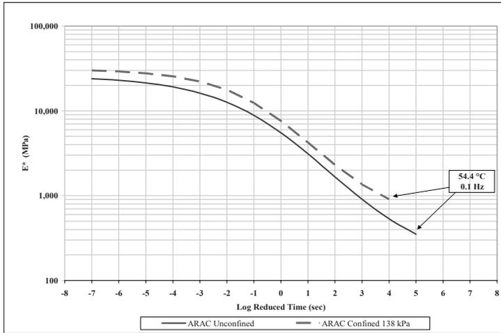
**Figure 2.** Dynamic Modulus Master Curves for ARAC Mixtures at Unconfined and Confined Conditions (138 kPa).
