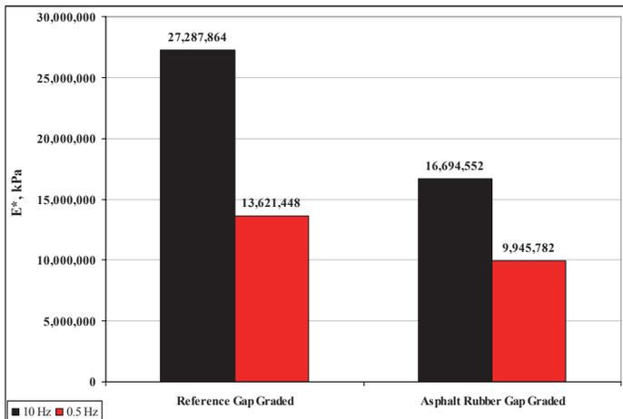
**Figure 4.** Comparison of Measured Dynamic Modulus E\* values at 4.4 °C for the Reference and the Asphalt Rubber Gap Graded Mixtures at 10 and 0.5 Hz
