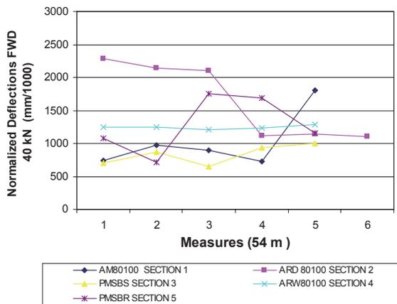
Figure 12. FWD center of plate deflections for each section
