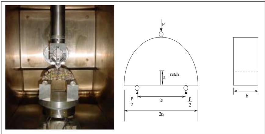
Figure 2. Set-up of Semi-Circular Bending Test
