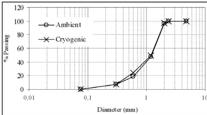
**Figure 3.** Grain size distribution curves of crumb rubber obtained from the ambient grinding and from the cryogenic processes
