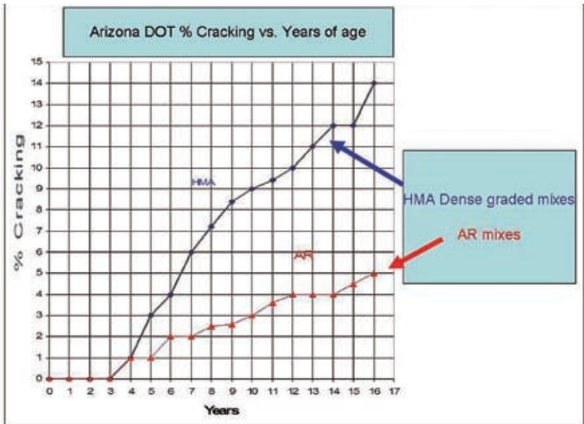
**Figure 12.** Percent cracking versus years of service for HMA and asphalt-rubber pavements
