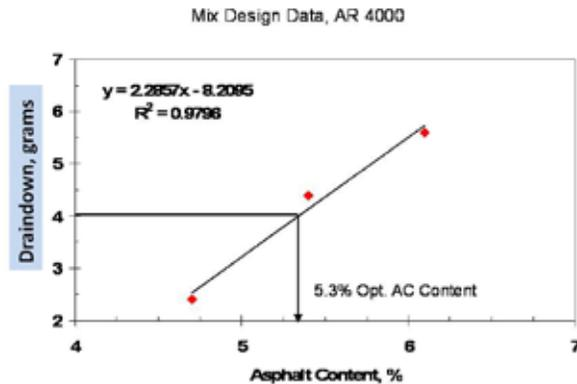
Figure 3. Selecting optimum binder content for open graded mix (Kc is 1.4)
