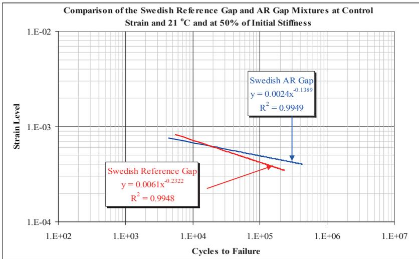
Figure 7. Comparison of Fatigue Relationships at 50% of Initial Stiffness
