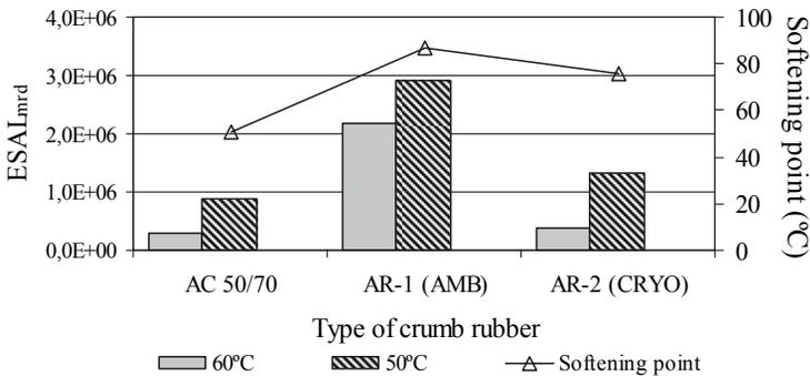
**Figure 10.** Results of RSST-CH tests for dense graded asphalt hot mixes
