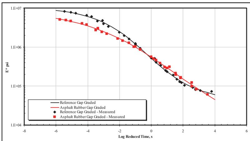
Figure 3. E\* Master Curves for Both Mixtures.
