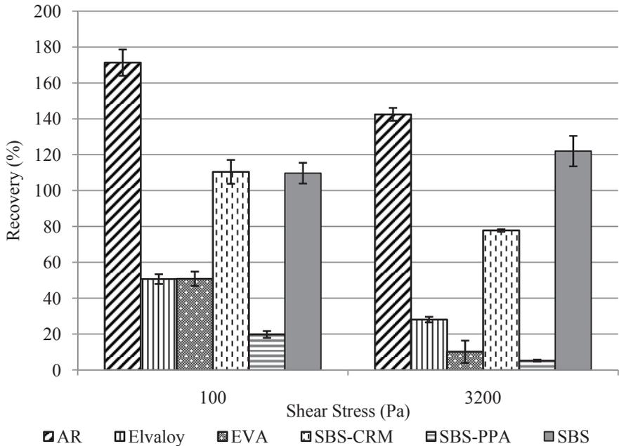
**Figure 3.** Percent recovery at 100 and 3200 Pa at 70°C
