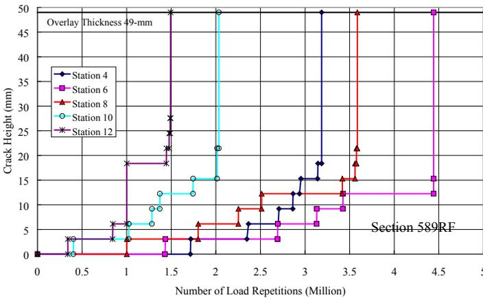
**Figure 19.** Evolution of height of crack tip with number of load repetitions for sub-sections of HVS section DGAC.
