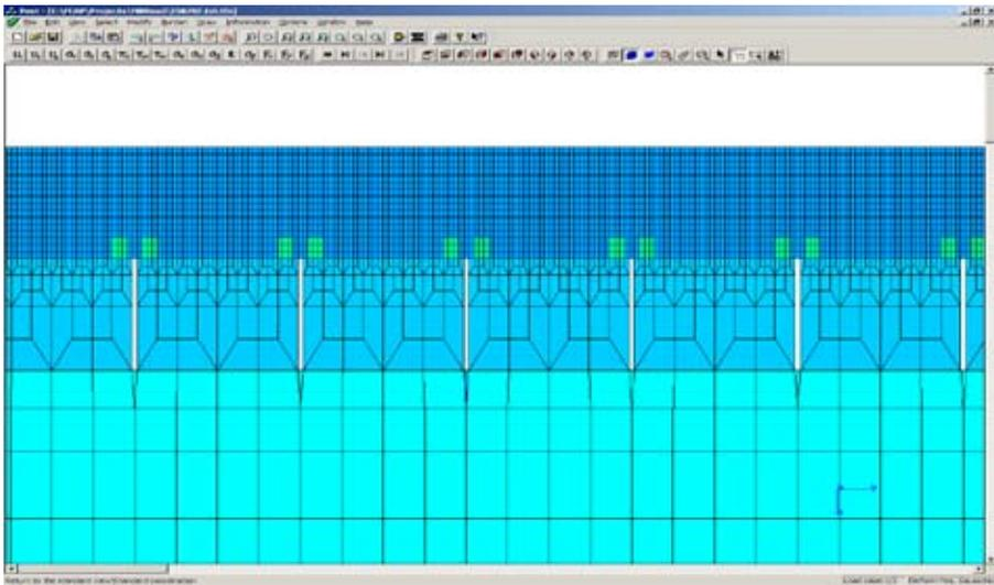
**Figure 18.** Close up look of the FEM mesh. The green blocks in the overlay around the tip of the underlying cracks indicate areas that are not subjected to damage. These blocks are necessary to force cracks to propagate upwards instead of sideways.
