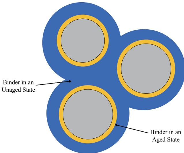
**Figure 4.** Increase of Air Voids Due to Aging and Decrease of Film Thickness
