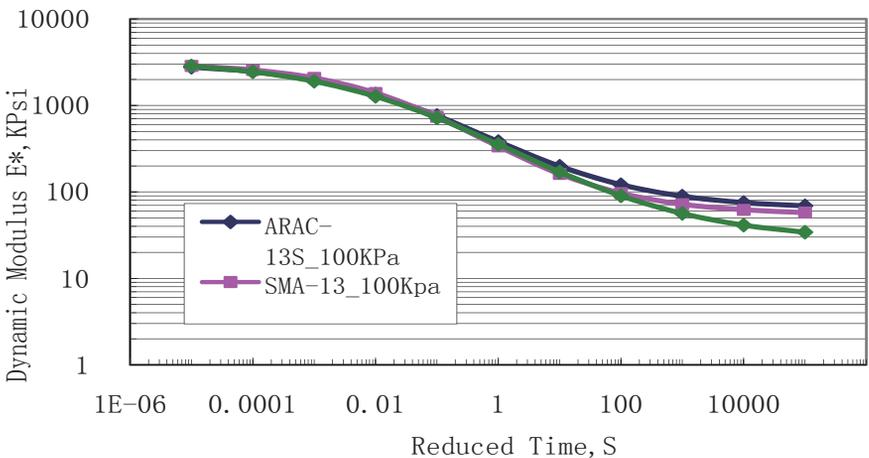
**Figure 2.** Dynamic Modulus Master Curve( 25°C, Confined, 100Kpa)
