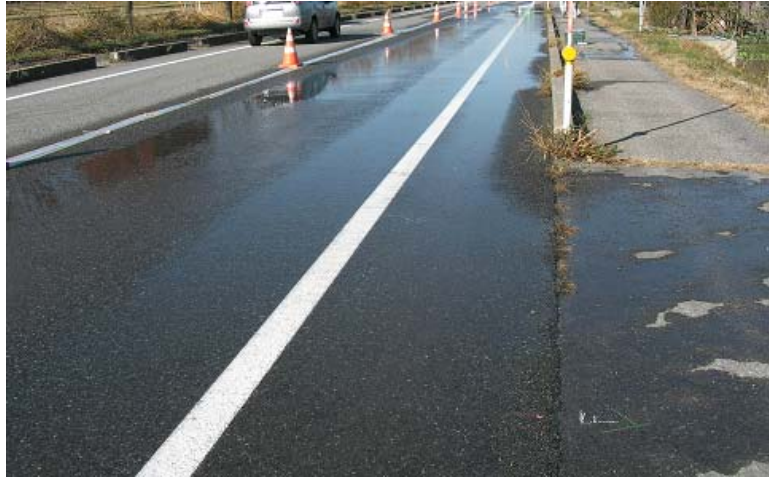
Photo 5 : Situation of the watering experiment after 50 months of service at Section B
