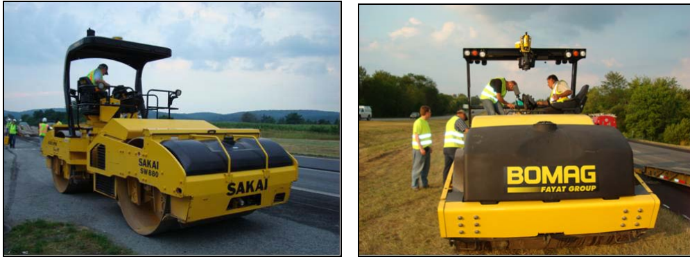
Figure 1: Sakai (left) and Bomag (right) Tandem Drum IC Rollers.
