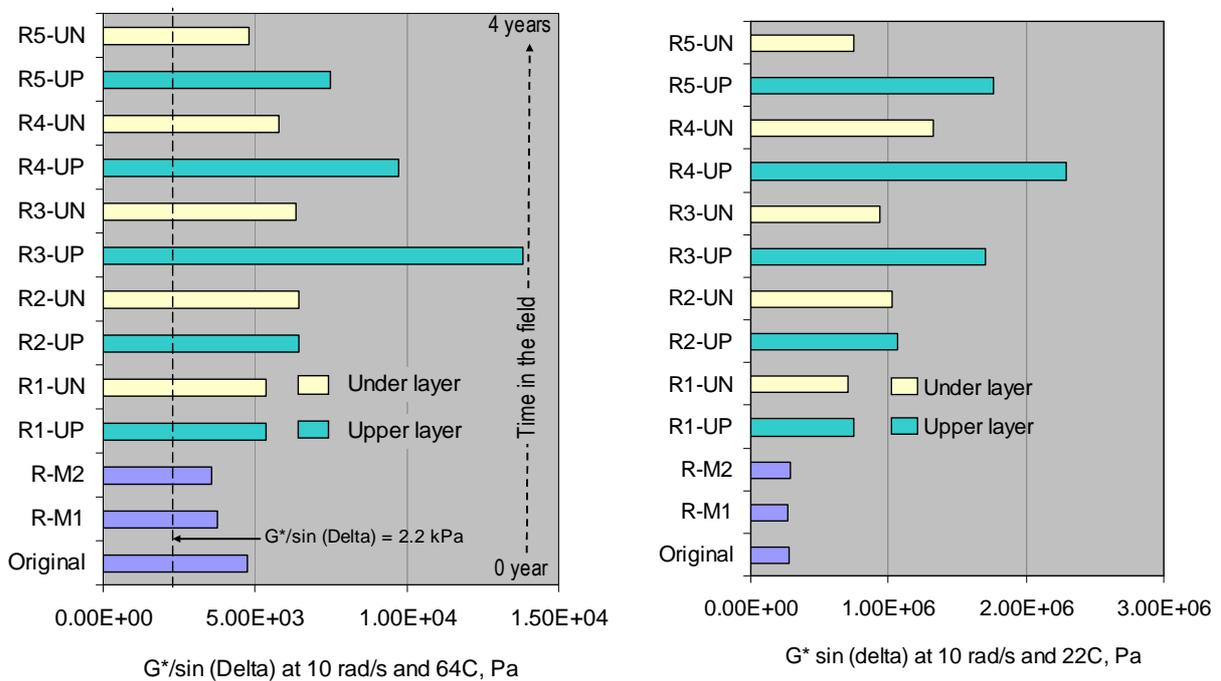
Figure 5: Rheological comparison according to the SHRP rutting and fatigue parameters
