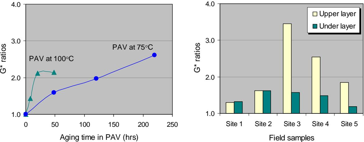
Figure 9: Comparison of the long-term ageing test PAV and the field aging
