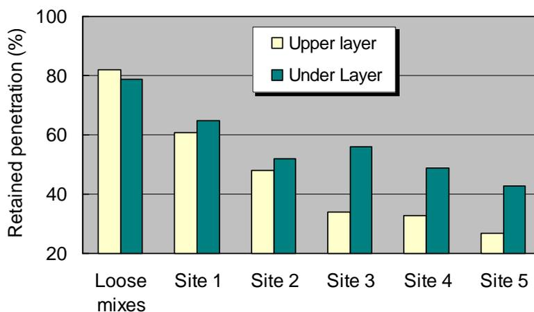
Figure 3: Retained penetrations of the recovered binder samples
