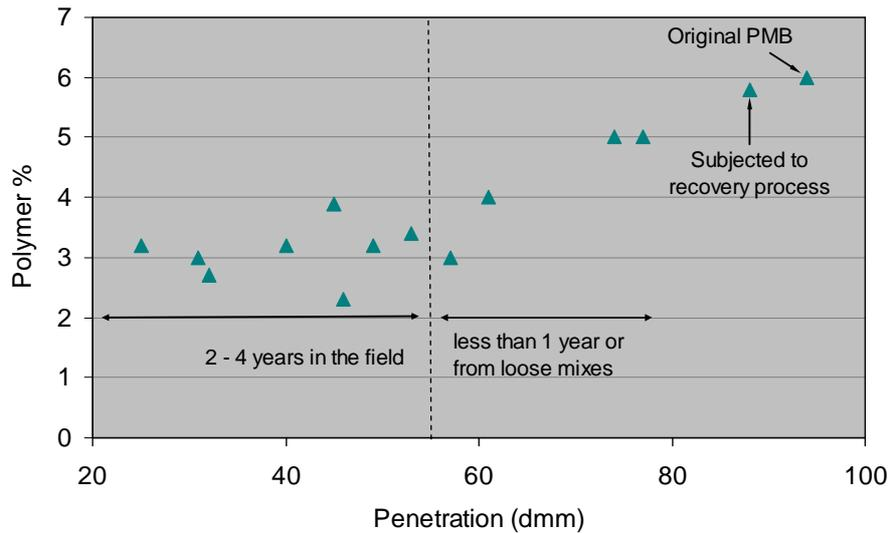
Figure 7: Polymer contents estimated by GPC *versus* penetration of the binders
