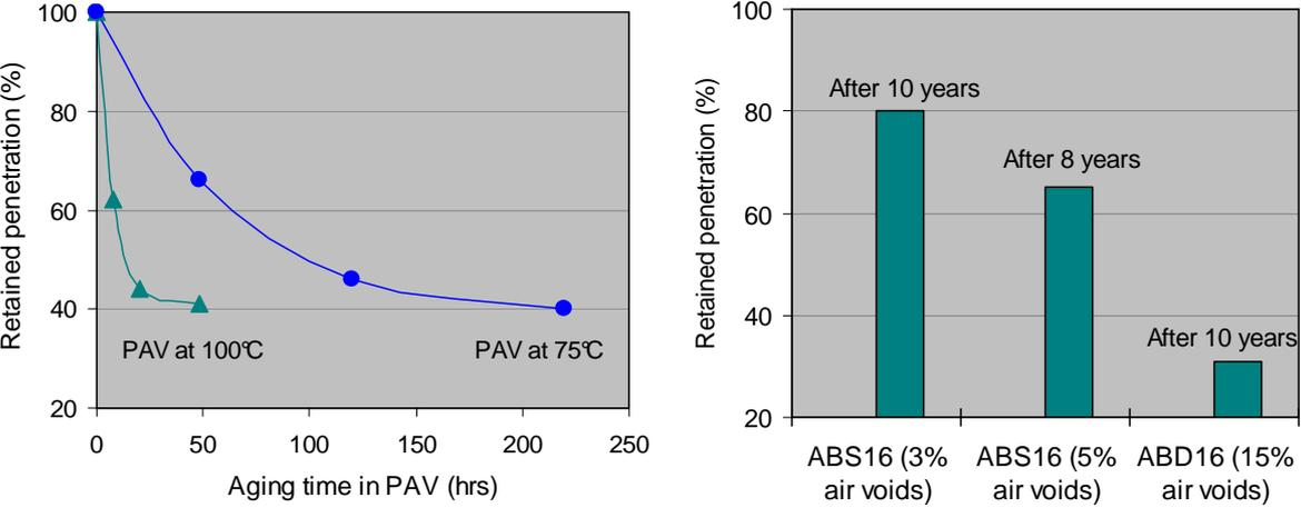
Figure 10: Comparison of PAV and the field aging of other mixes
