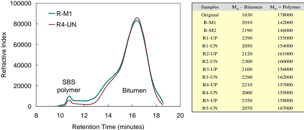
Figure 6: Examples of GPC chromatograms and the measured molecular weights
