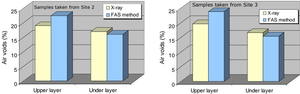
Figure 2: Comparison of air void contents measured by X-ray tomography and FAS method
