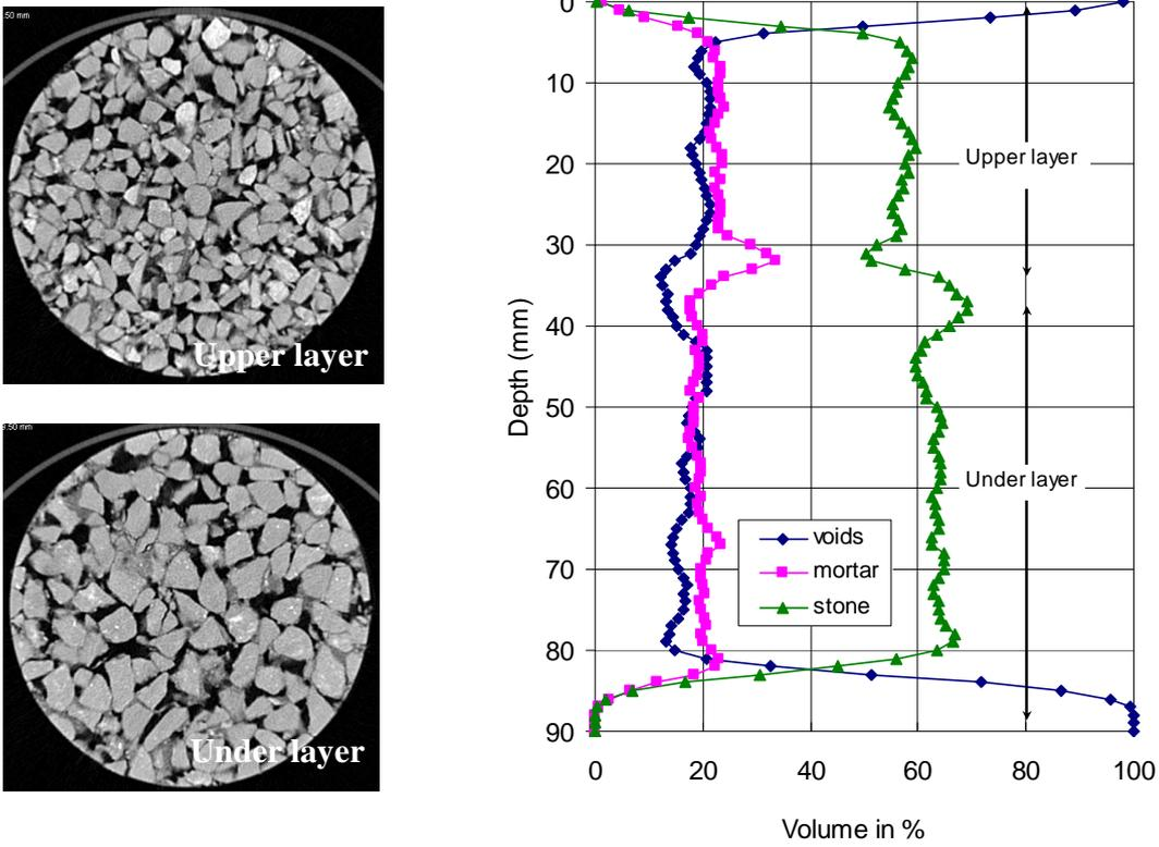
Figure 1: X-ray tomography analysis of a field core
