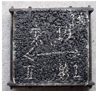
Figure 5: A rut specimen fabricated in laboratory
