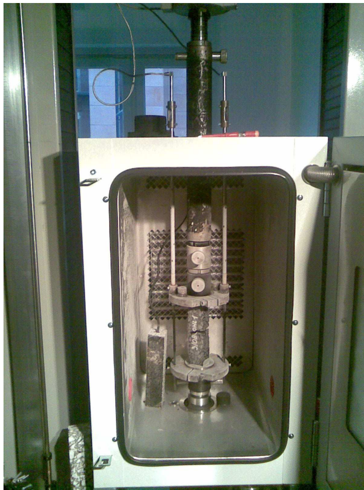
Figure 3: Apparatus for testing asphalt specimens at low temperatures in the thermo-static chamber at ZAG
