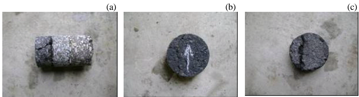
Figure 4: Core sample taken at longitudinal crack level. (a) The first interface is detached whereas the first layer is cracked straight down. (b) View from above the wearing course. (c) View from below the wearing course.
