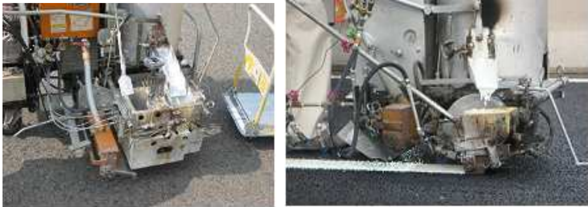
Figure 4: Thermoplastic paint applicator, Spray type (Left), Screed type (Right)
