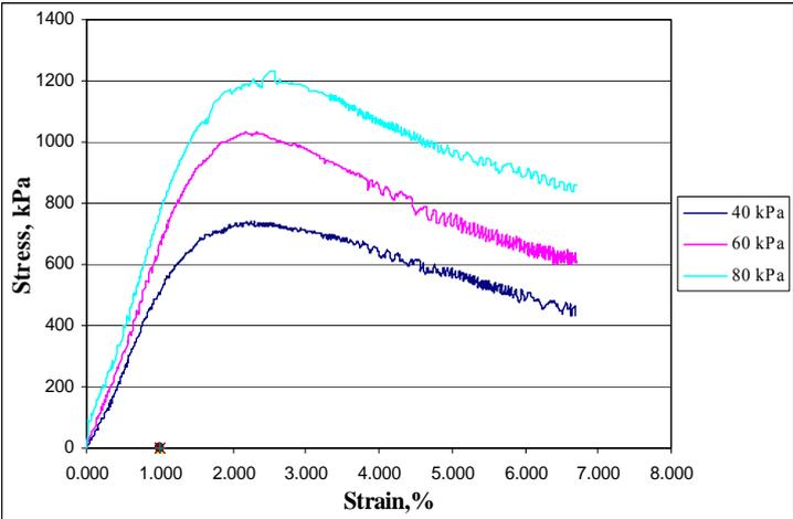
Figure 6: Triaxial shear test results.
