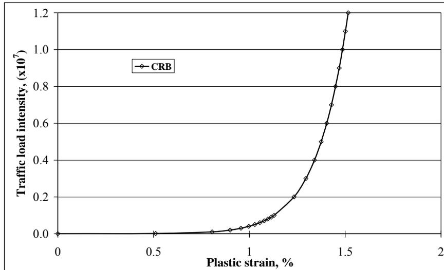
Figure 7: The amount of traffic compared with plastic strains.
