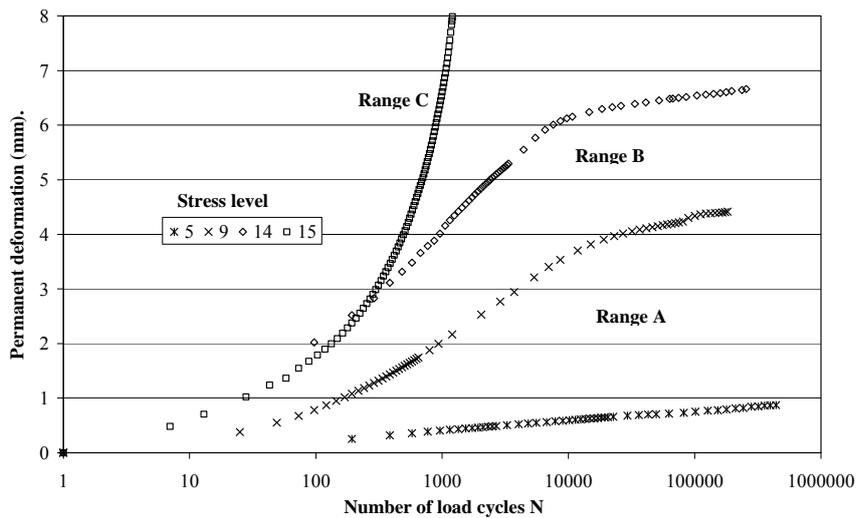
Figure 4: Permanent deformation versus number of load cycles (N).
