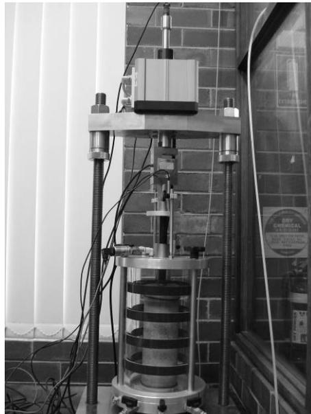
Figure 2: The repeated loads triaxial apparatus.
