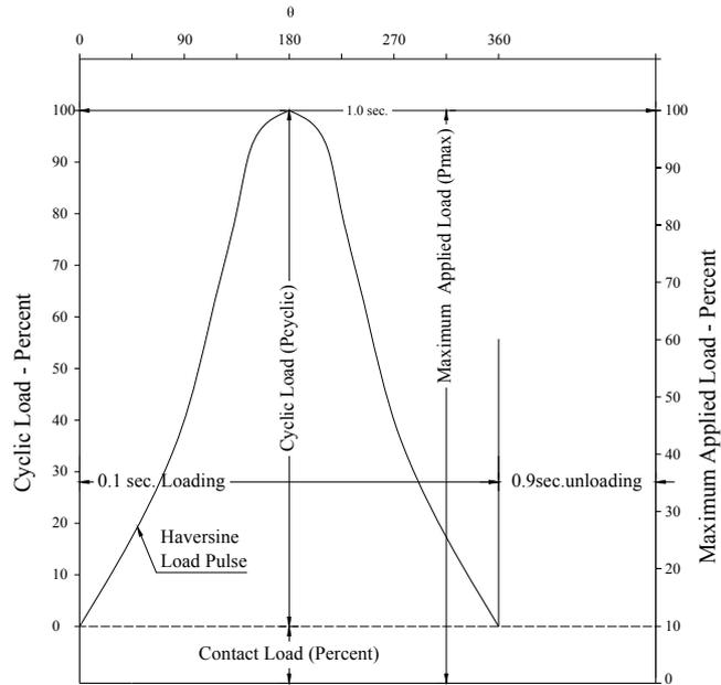
Figure 3: The vertical loading waveform.
