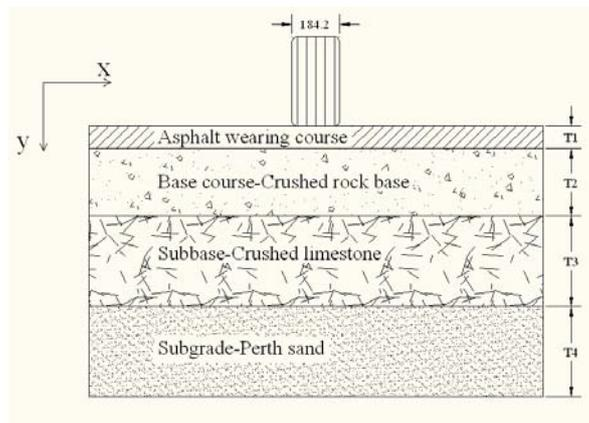
Figure 1: Pavement structure diagram.
