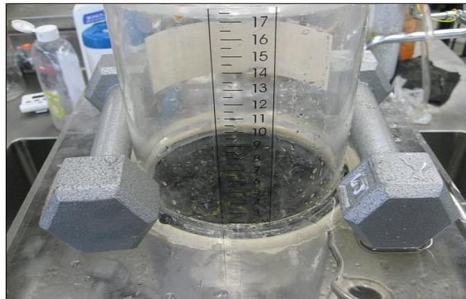
Figure 4: CPATT Gilson permeameter apparatus (Schaus 2007).
