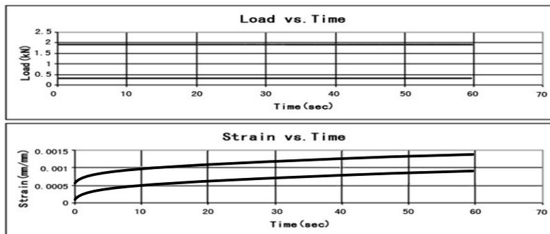
Figure 3: Graphs for dynamic modulus testing.
