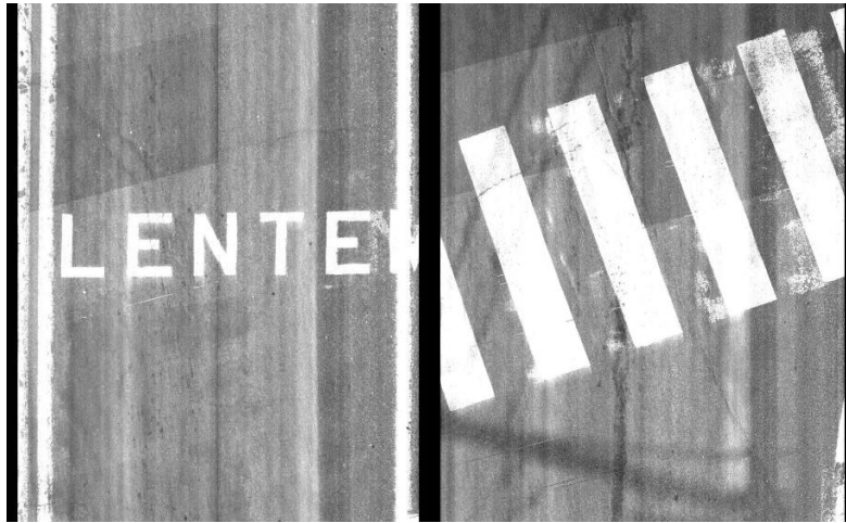
Figure 5: LCMS images of painted lane marks
