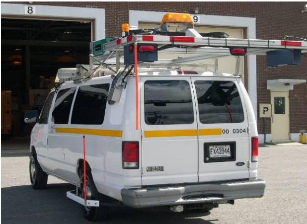
Figure 1: Photo of the LCMS on the MTQ Inspection Vehicle
