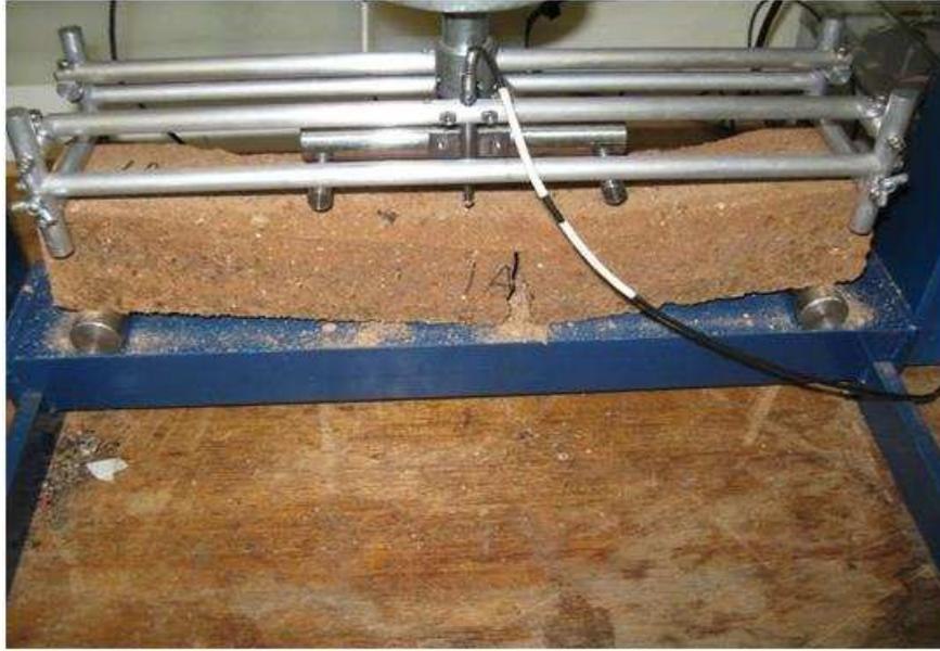
Figure 4: Typical specimen failure mode
