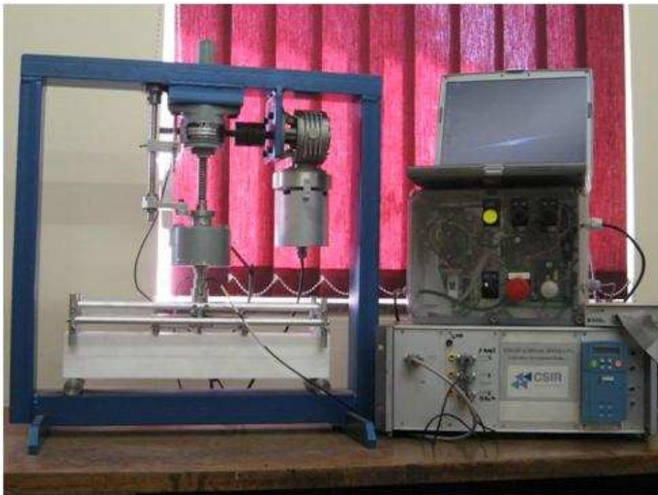
Figure 1: Strain-at-break-device set up
