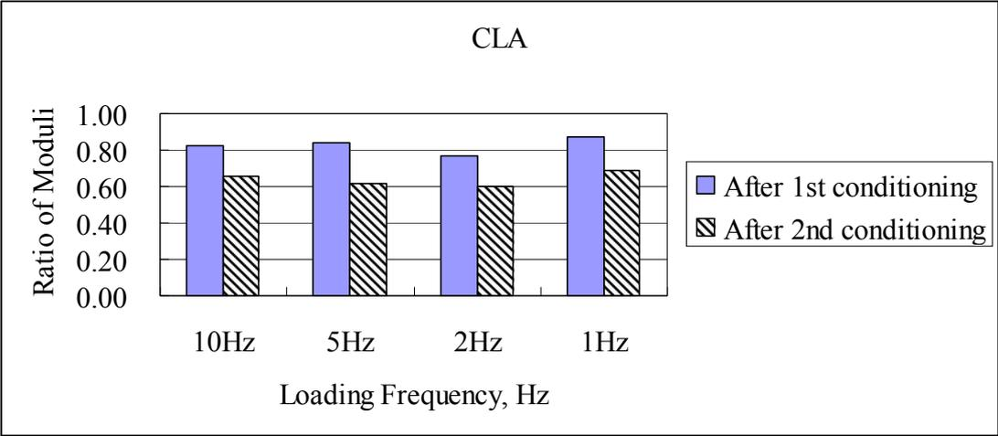
Figure4: Ratio of moduli for different frequencies for CLA mix.
