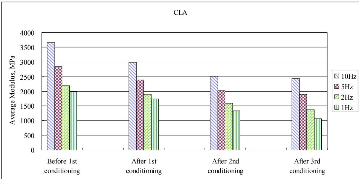
Figure2: Average modulus for different frequencies and different conditioning levels for the CLA mix.
