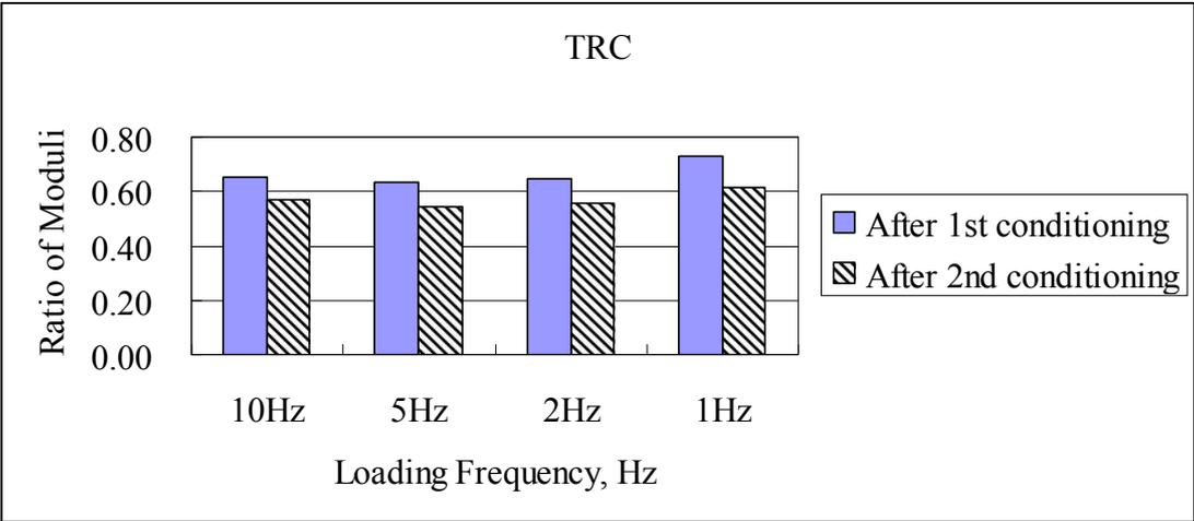
Figure3: Ratio of moduli for different frequencies for TRC mix.
