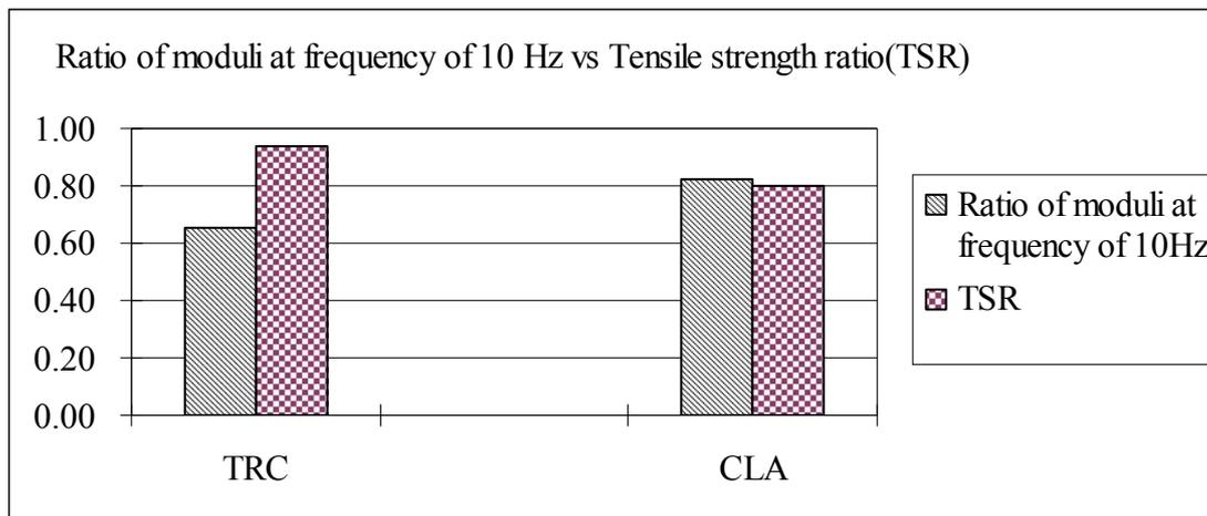
Figure6: Ratio of moduli at frequency of 10 Hz versus tensile strength ratio (TSR).
