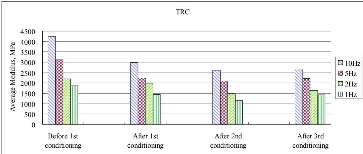
Figure1: Average modulus for different frequencies and different conditioning levels for the TRC mix.
