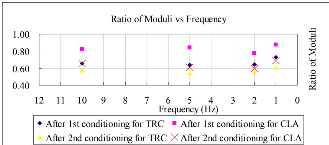
Figure5: Ratio of moduli at different frequencies.
