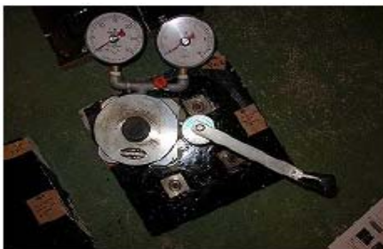
Photo 7: Bond Strength Test under Way
