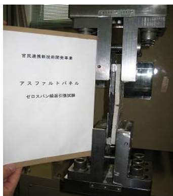
Photo 4: Zero-span Test under Way
