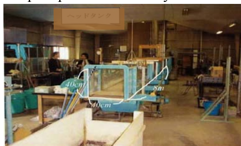
Photo 1: Experimental Measurement of Roughness Coefficient
