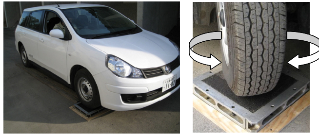
※ contact pressure of tire : 0.37(N/mm 2 ) , handle operation : left and right one full turn
