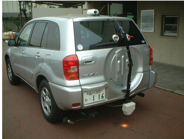
Photo 1: Measurement vehicle of tyre/road noise
