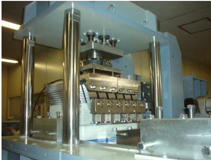
Figure1: Large-scale direct simple shear apparatus and its constrained conditions.
