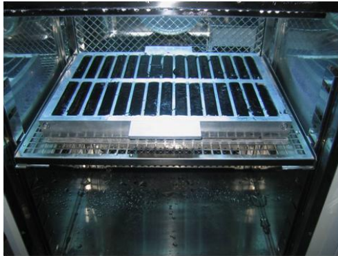
Photo 5: Binder specimen for accelerated weathering test.
