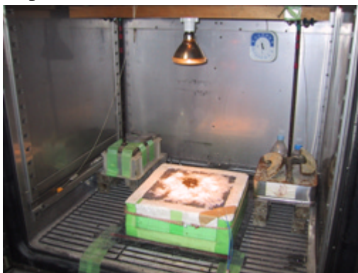
Photo 3: Confirmation of snow-melting using indoor irradiation test
