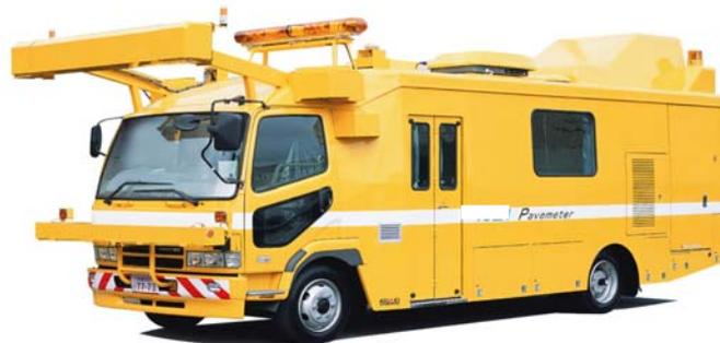
Photo 1: New road surface-measuring vehicle “Pavemeter Ver. IV”
