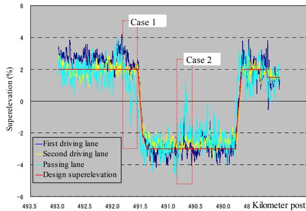
Figure 6: Detecting points of puddle formation from cross grade diagrams
