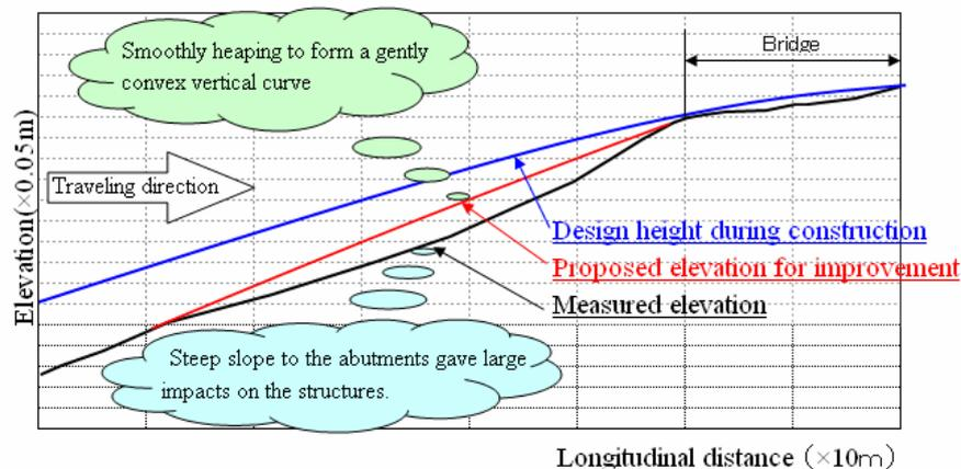
Figure 5: Determination of the present longitudinal profile and a proposed improvement plan
