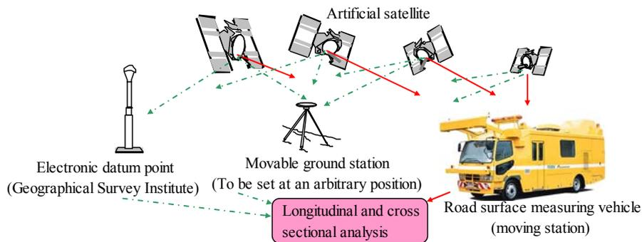
Figure 3: Kinematic GPS measurement using the road surface-measuring vehicle
