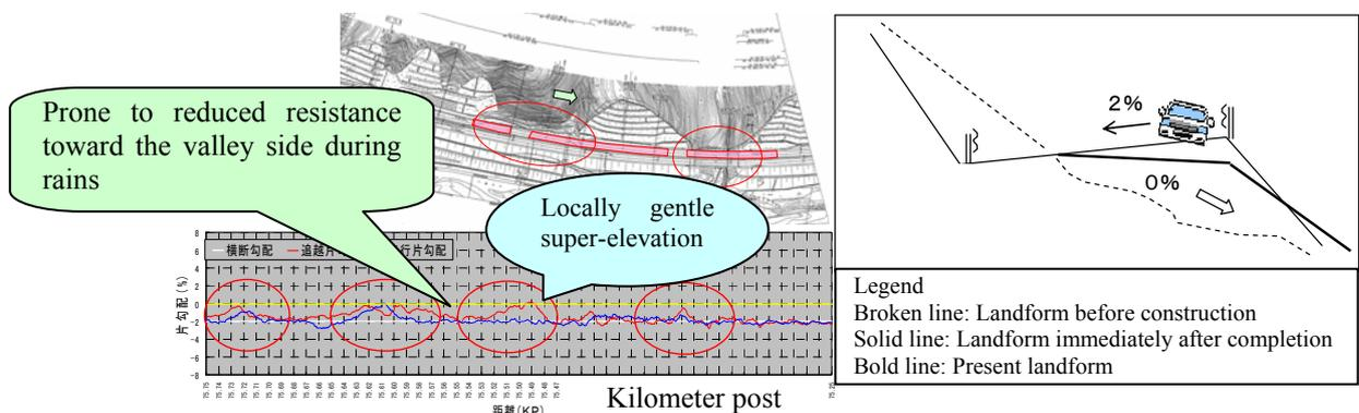
Figure 8: Assessing driving safety by measuring cross super-elevation
