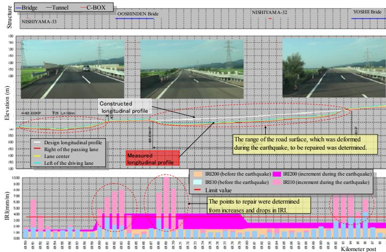
Figure 9: Longitudinal profile and IRI values (Comparison between before and after the earthquake)
