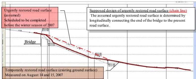
Figure 10: Temporary and emergency repairs to road surface
