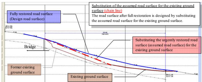
Figure 11: Emergency repairs and fully restored road surface
