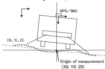
Figure 4: Schematic diagram of three-dimensional data link
