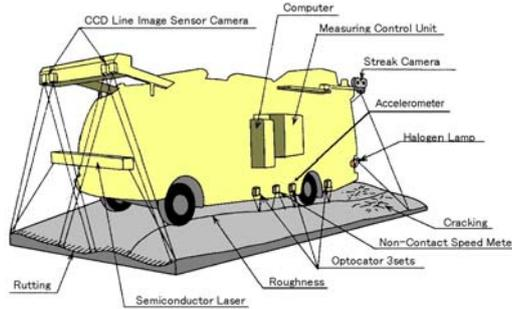
Figure 1: Schematic diagram of the “Pavemeter Ver. IV”
