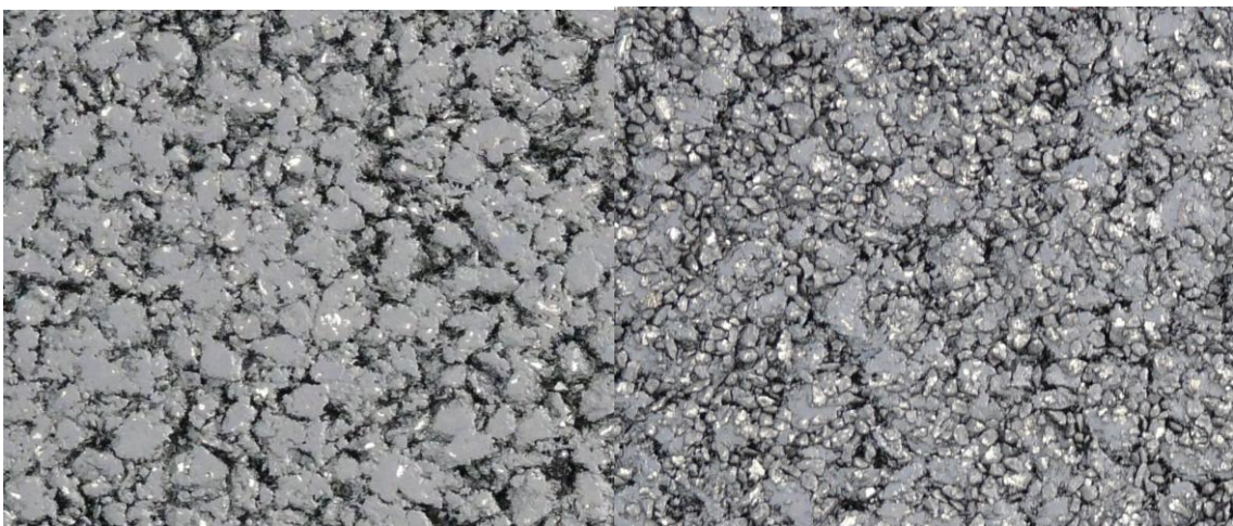
Figure 3: Close-up of 0/14mm before (left) and immediately after gritting (right)
