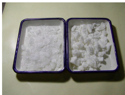
Figure 1: Appearance of solid epoxy resin (left: base compound; right: curing agent)
