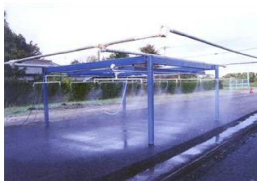
Figure 2: View of rainfall simulation test equipment
