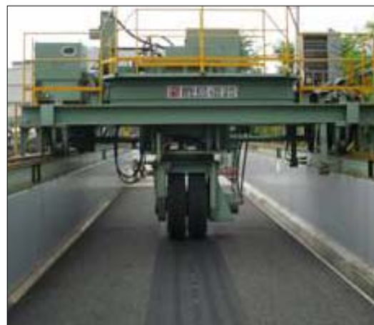
b) run situation by accelerated loading device
