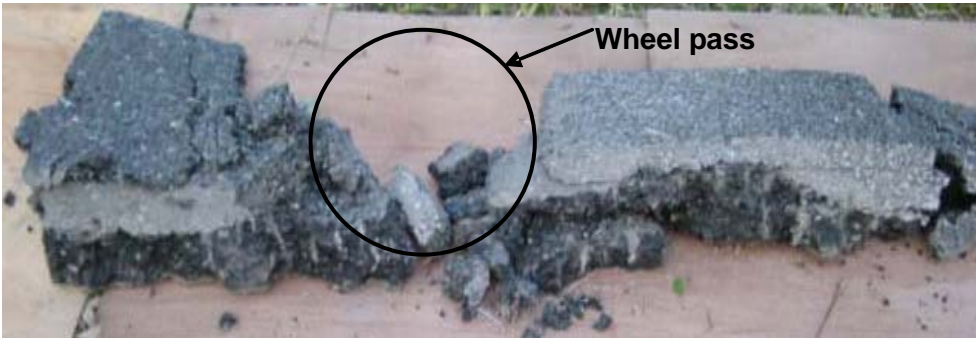
Photo2 Cut specimen after accelerated loading test
