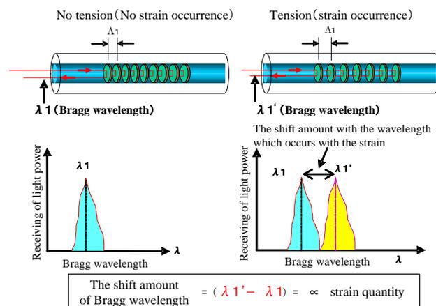
Figure 2 The principle of the FBG type optical fiber sensor
