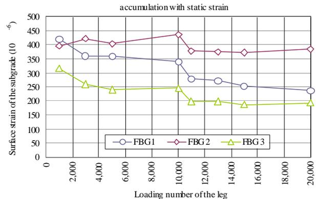
Figure 5 The change of the static strain of the subgrade to the loading number of the gear
