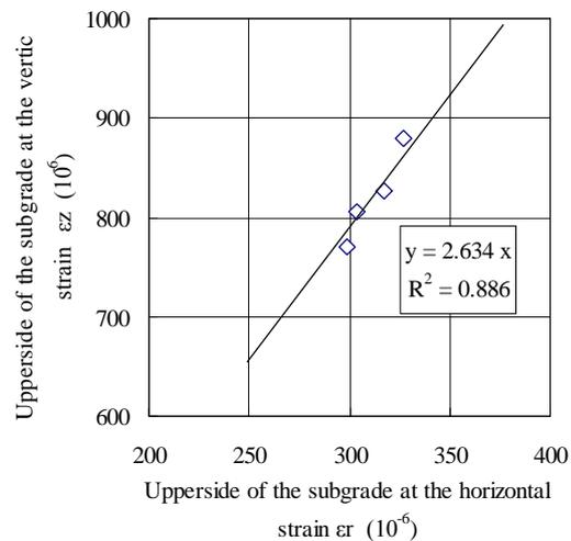
Figure 14 The comparison between the calculated and measured strain values (After 5.000 times)
