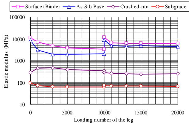
Figure 11 Relation between the estimated elastic modulus and the loading number of gear
