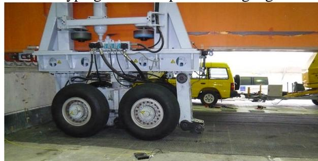
Photo 2 The overview of this moving load equipment
