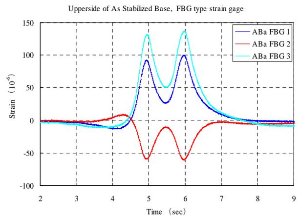
Figure 7 The strain wave which was measured with the FBG type strainmeter in the upperside of the asphalt stabilized base by the 3,000th moving load test
