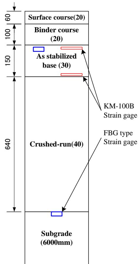
Figure 1 Pavement structure of runway (LA-1)
