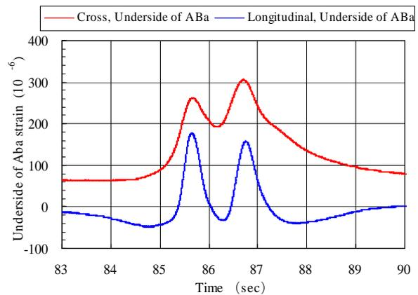
Figure 9 The strain way with the ground-coupled strain sensor which was laid to the crossing direction and the longitude direction in the underside of the asphalt stabilized base
