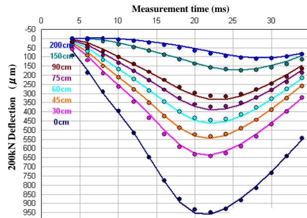
Figure 16 The comparison between deflections at 5000 passes measured by FWD and the deflection waveform of DBALM that was backcalculated by dynamic FEM analysis
