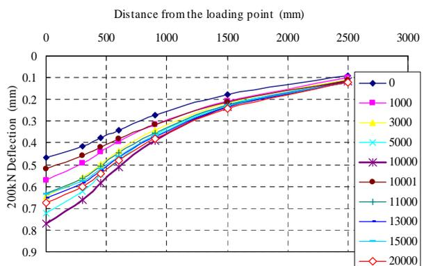
Figure 10 The deflection basin which was measured loading number of the gear
