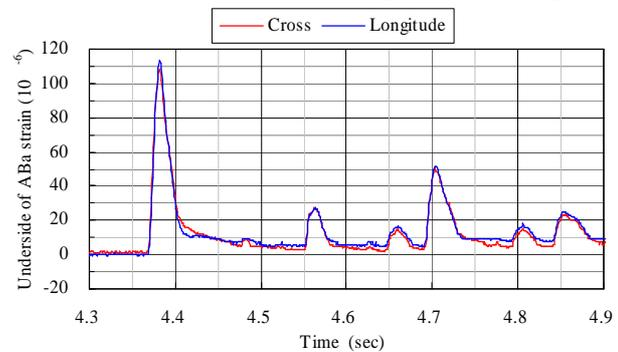
Figure 12 The strain to the longitude direction and the cross direction in the asphalt stabilization underside at the FWD load
