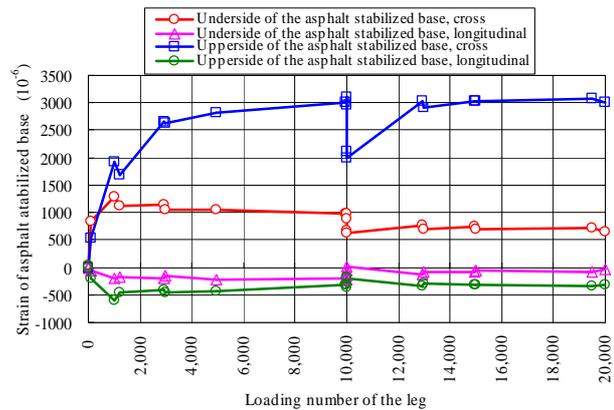
Figure 6 The change of the static strain of the upperside and the underside in the asphalt stabilized base layer to the loading number of the gear load
