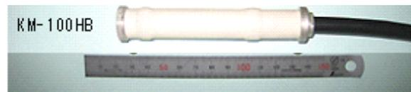
Figure 3 The structure and the size with KM type ground-coupled strain gauge
