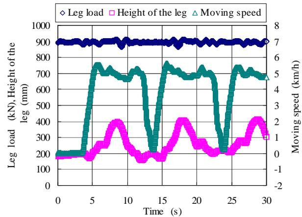
Figure 4 The Relationship between the actual gear load and the moving speed
