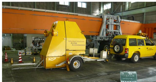
Photo 3 This place implemented deflection measurement at the time of 196kN load using the FWD for the airport on the strain gauge which was laid in the pavement
