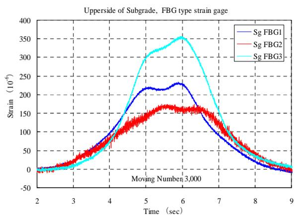
Figure 8 The strain wave by the moving load test at 3,000th with the FBG type strainmeter to have installed in the upperside of the subgrade
