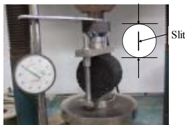
Figure 5: Splitting test of several specimen (test temperature:20°C)
