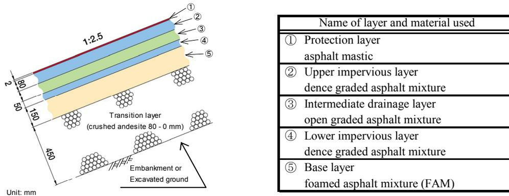
Figure3: Configuration of asphalt facing
