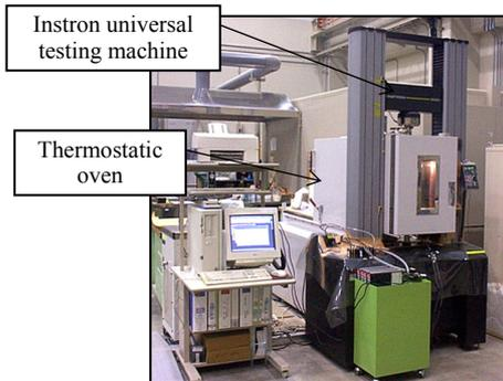
Photograph2: Full view of the testing system
