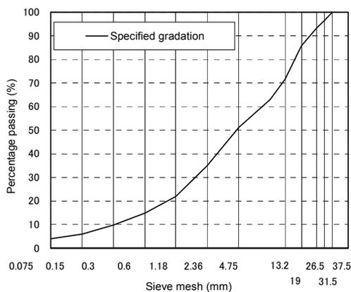
Figure5: Specified gradation
