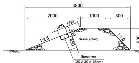
Figure6: Condition of the test
