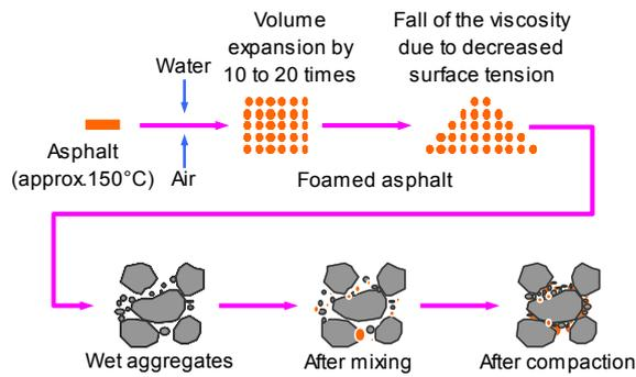
Figure4: Fundamentals of foamed asphalt and the manufacturing process of FAM
