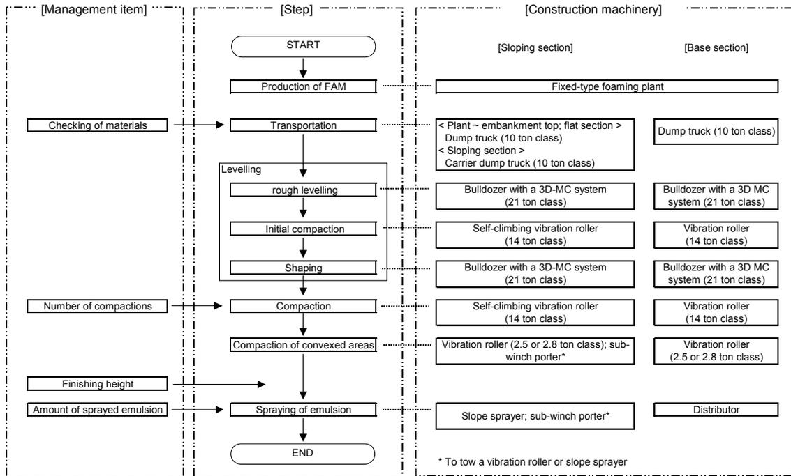
Figure11: Construction flow of the base layer and construction machinery to be used
