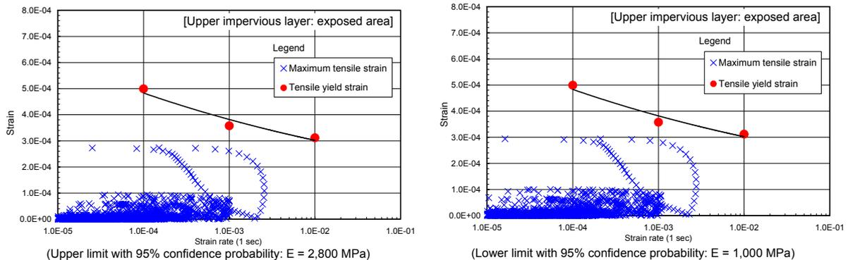
Figure8: Safety evaluation results (upper impervious layer)
