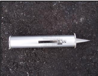
Photograph5: Yamanaka-Type Soil Hardness Meter
