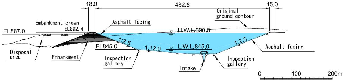
Figure2: Standard cross-section of the upper reservoir (A – A)
