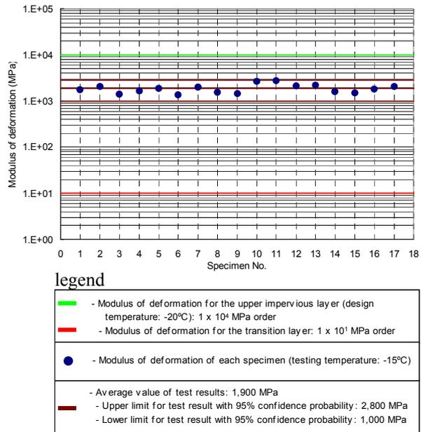
Figure7: Indirect tensile test results
