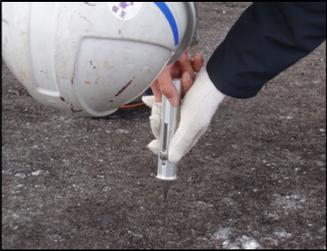
Photograph6: Measuring of the hardness
