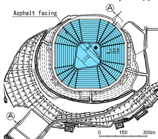
Figure1: Plan of the upper reservoir
