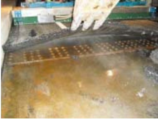
Photo 6: Removal Scene (Sufficient Heating) Photo 7: Asphalt Mixture Removed
