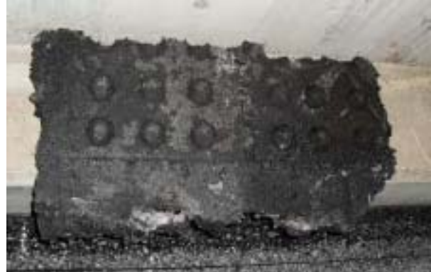
Photo 6: Removal Scene (Sufficient Heating) Photo 7: Asphalt Mixture Removed
