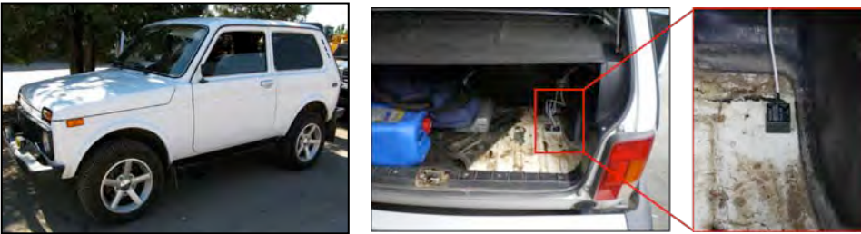
Figure7: Measurement system in Kyrgyz; measurement vehicle of Russian make, installation of an accelerometer
