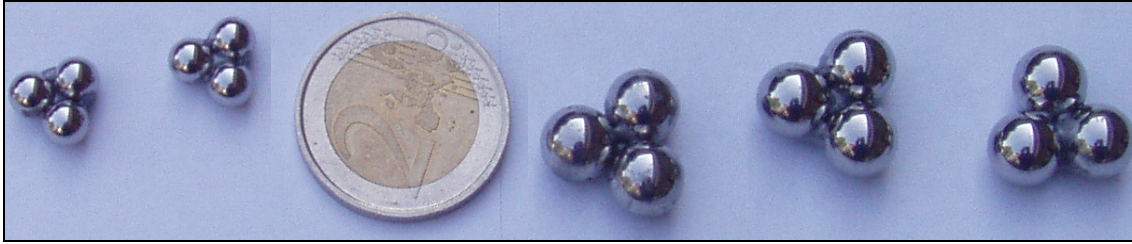
Figure 8: Steel clumps of spheres used in the second research step
