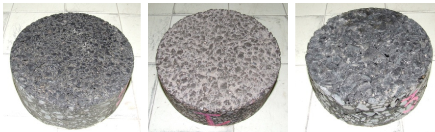
Figure 10: Conventional, SMA and draining samples
