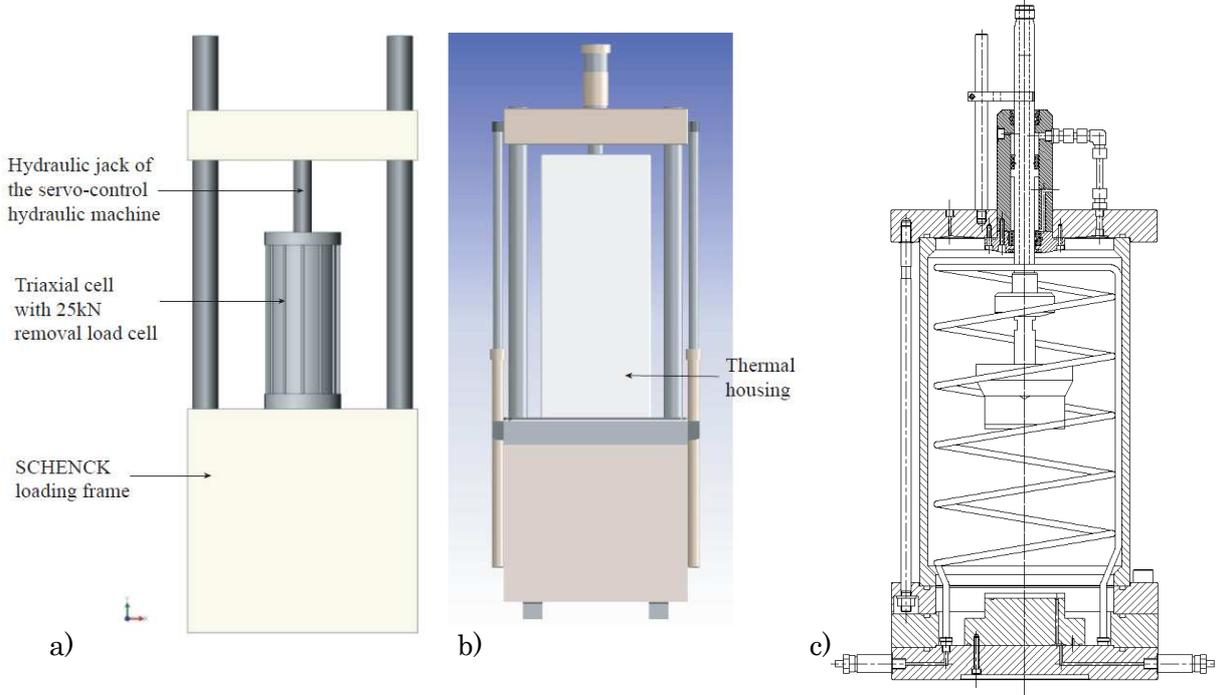
Figure 3: Schematic view of the triaxial testing equipment without (a) and with (b) the thermal chamber and schematic view of the triaxial cell (c)
