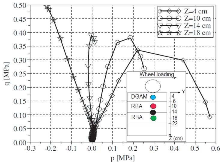
Figure 2: Stress paths at different depths  $z$  in bituminous layers
