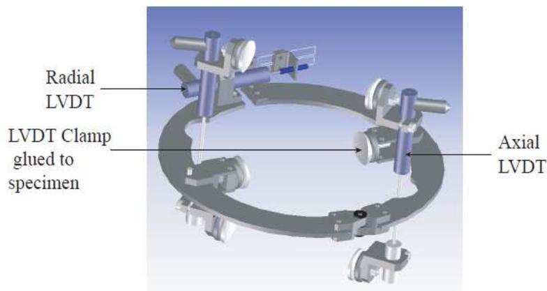
Figure 4 : Schematic view of the axial and radial LVDT sensors
