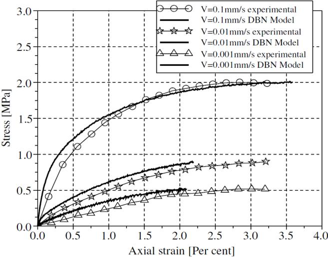
Figure 7 : Experimental creep test results at 20°C, for 3 different strain rates and corresponding predictions obtained with the 15-elements DBN model
