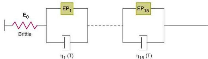
Figure 5 : Structure selected for the discrete DBN model (Olard and Di Benedetto, 2005)
