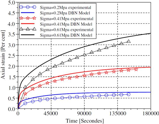
Figure 8 : Experimental creep test results at 10°C for 3 different stress levels and corresponding predictions obtained with the 15-elements DBN model
