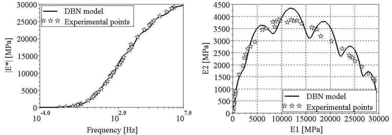
Figure 6 : Comparison of complex moduli obtained by means of the discrete (15 elements) DBN model and experimental results at 20°C.
