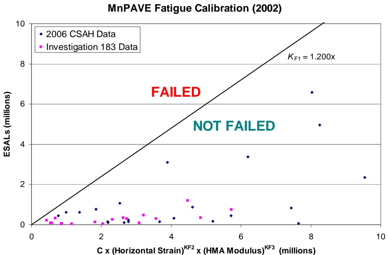
Figure 2: Validation of MnPAVE 2002 Fatigue Model (for up to 7 million ESALs).
