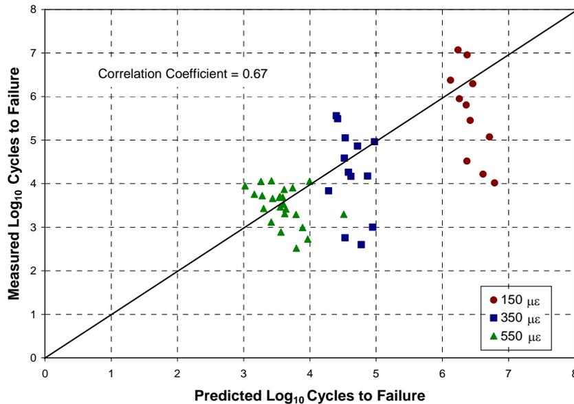
Figure 1: Measured versus predicted fatigue failure for aged field samples using original DoD fatigue criterion (Equation 1).
