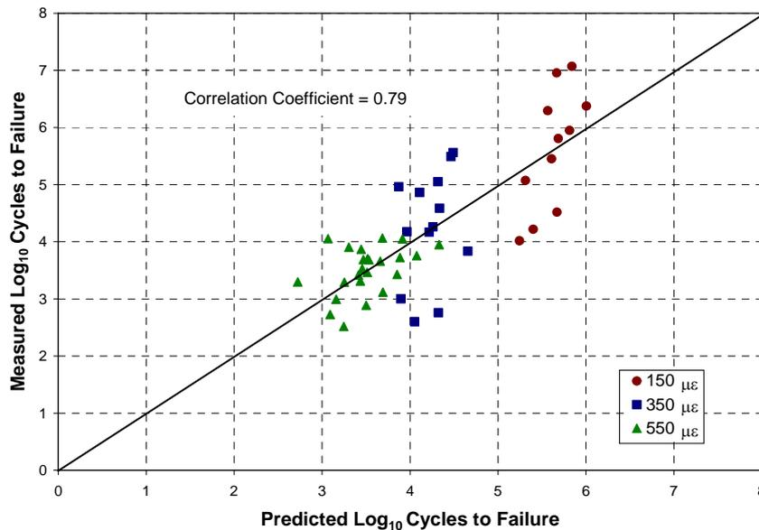
Figure 2: Measured versus predicted fatigue failure for aged field samples using Equation 3.
