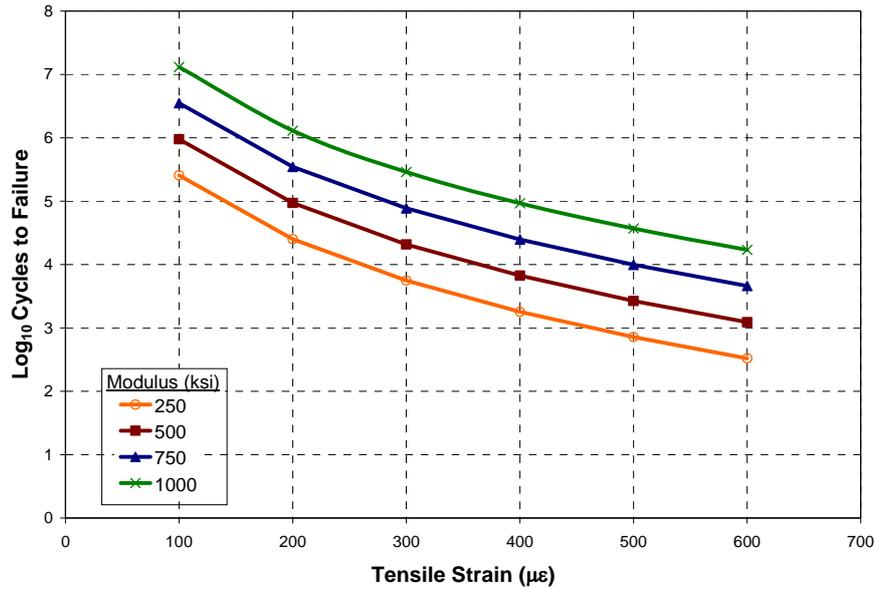
Figure 3: Fatigue evaluation curves for aged HMA based on Equation 3.
