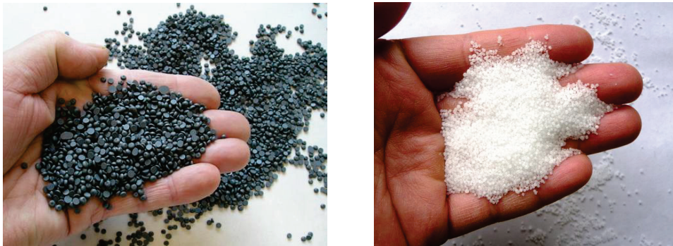
Figure 1: Modified sulfur pellets (left) and compaction agent (right) used in sulfur-modified WMA.
