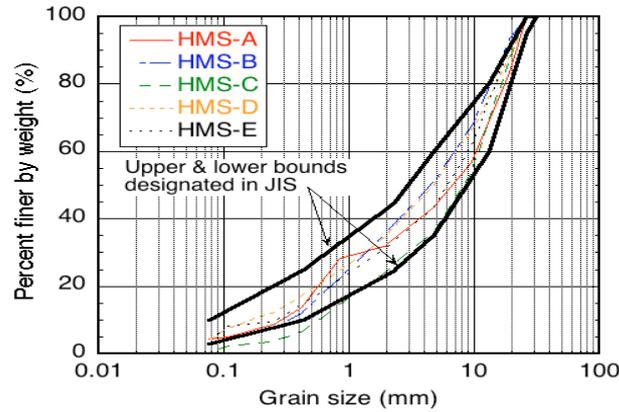
Figure 1: Grain size distributions of five types of hydraulic, graded iron and steel slag
