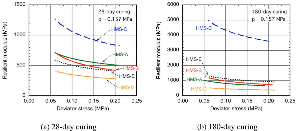
Figure 8: Relationships of resilient modulus with deviator stress for five HMS
