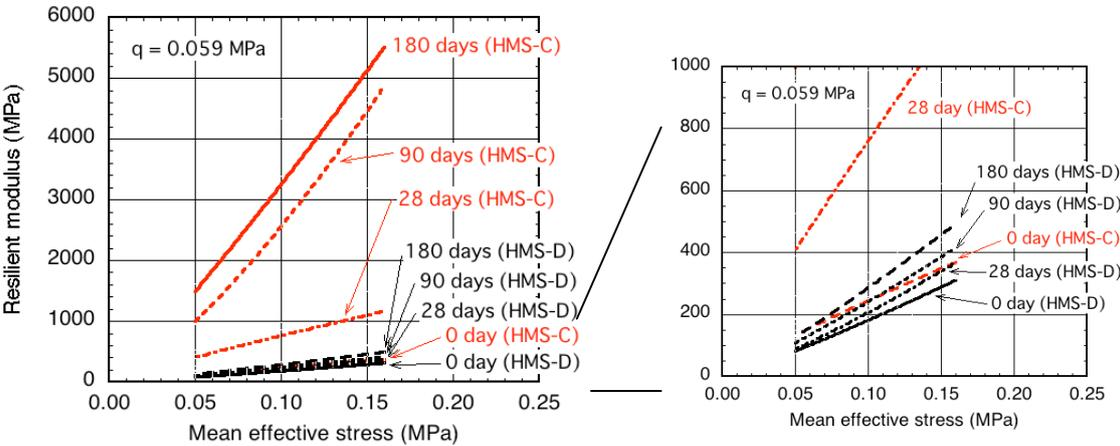
Figure 7: Relationships of resilient modulus with mean effective stress for HMS-C and HMC-D at curing time from 0 to 180 days
