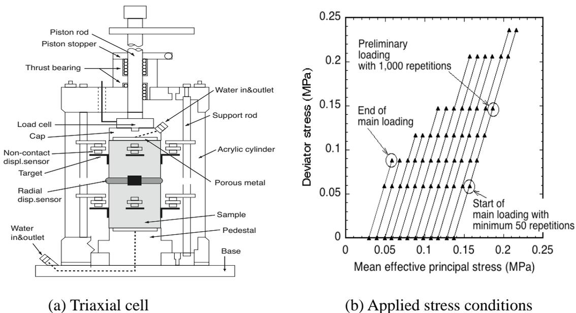
Figure 5: Triaxial cell and applied stress conditions for repeated loading triaxial compression tests
