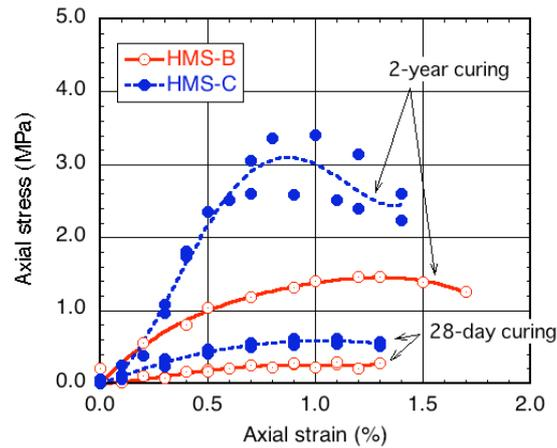
Figure 3: Relationships of axial stress with axial strain for HMS-B and -C at 28-day and 2-year curing
