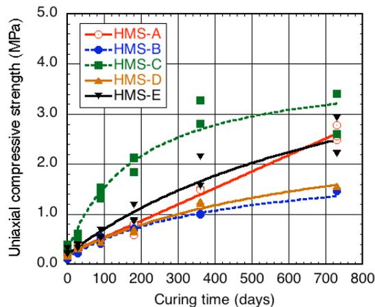
Figure 4: Relationships of uniaxial compressive strength with curing time
