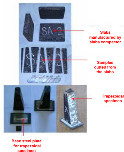
Figure 1: Preparation of trapezoidal specimens for stiffness modulus assessment.
