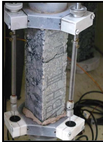
Figure 6: Specimen (ACL 16 + 3% Licomont) after test termination.
