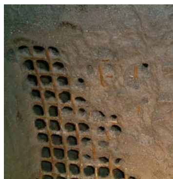
Photo3: State of Trommel after Heating Experiment (140°C)
