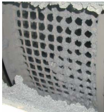
Photo2: State of Trommel after Heating Experiment (160°C)
