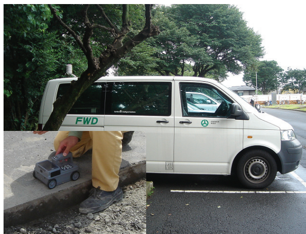
Figure 3: Falling weight deflectometer and electromagnetic waves
