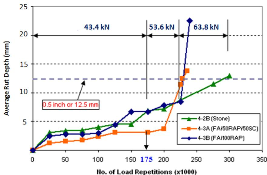
Figure 2: Measured rut depths on test sections
