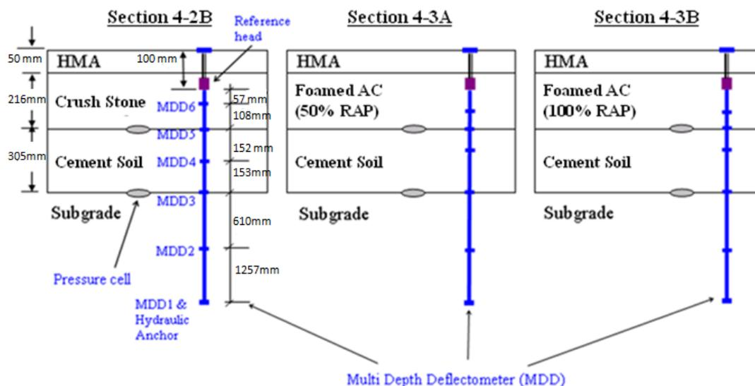
Figure 1: Pavement structures and instrumentation layout of APT test sections
