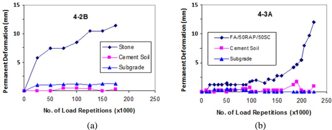
Figure 5: MDD measured permanent deformations
