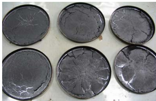
Figure 1: The asphalt specimen after UV radiation aging test
