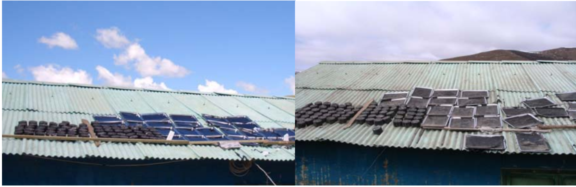
Figure 2: Before field UV aging Figure 3: Seven months after field UV aging
