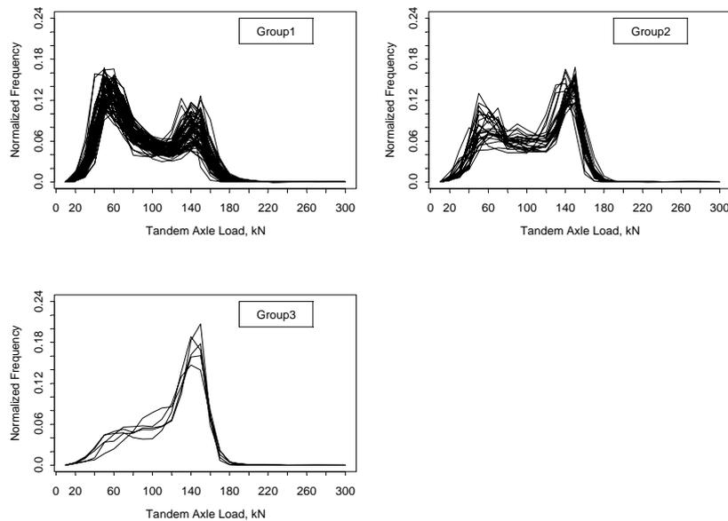
Figure 1: Tandem axle load spectra in each group.
