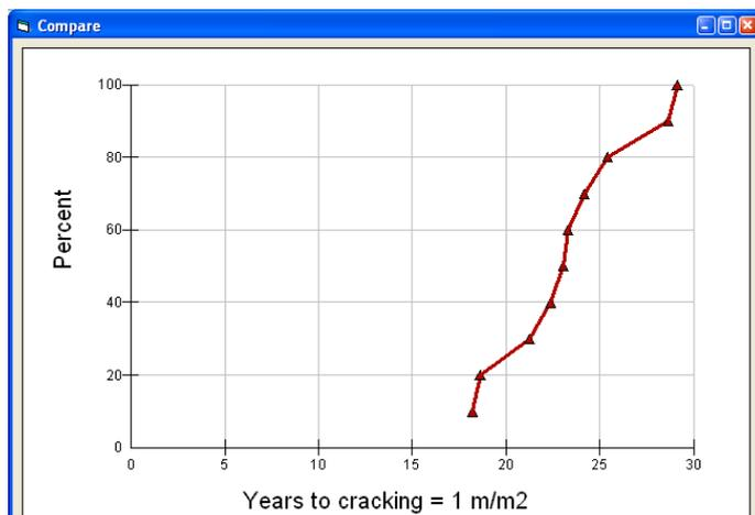
Figure 3. Percent of wheelpath cracked as defined by time to threshold cracking in each sub-section of project.
