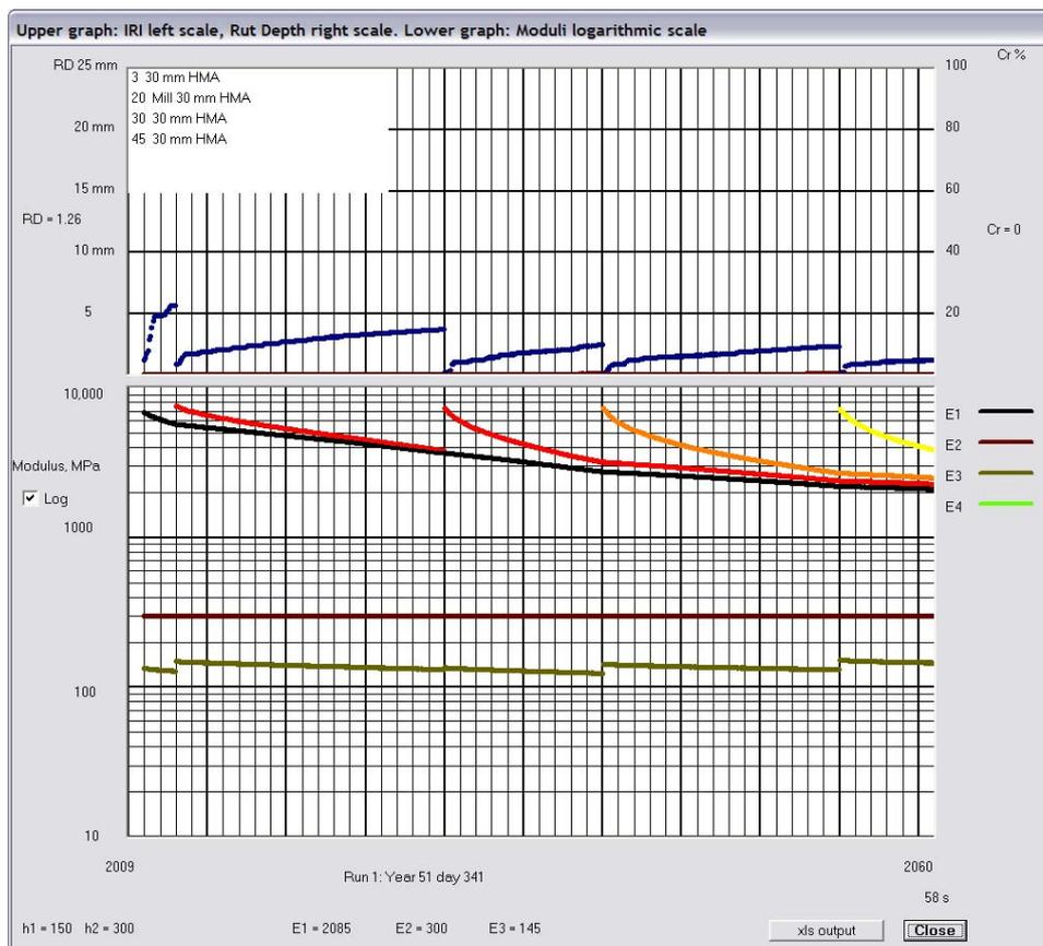
Figure 4. CalME simulation following a PPP strategy using 30-mm HMA. The maintenance activities are listed at the top left corner of the window. The first overlay occurred at year 3 and was triggered by 7-mm of total rut, the second overlay was triggered by age of the wearing course (17 years), the third, fourth and fifth overlays
