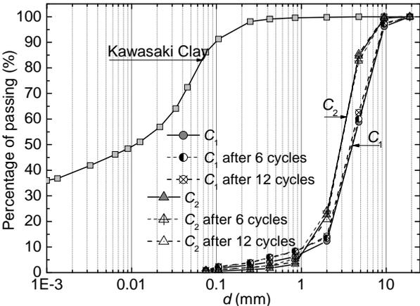
Figure 2: Grading curves of original Kawasaki clay and CTGS
