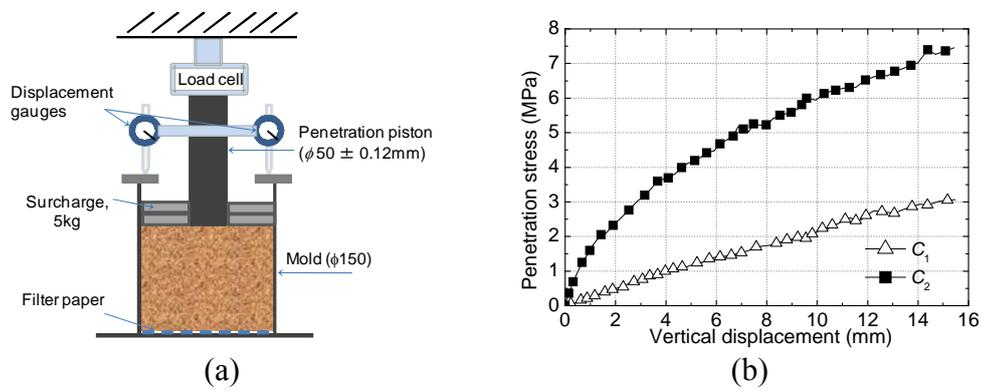
Figure 4: (a) CBR test (b) stress-penetration displacement curves
