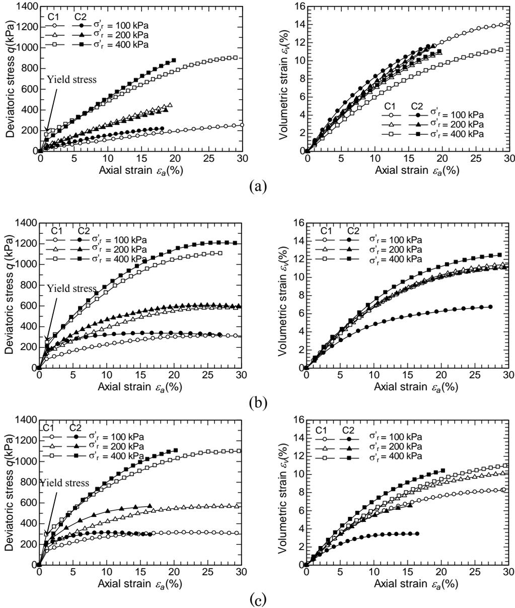
Figure 6: Deviatoric stress and volumetric strain versus axial strain at different confining pressures (a) Loose specimens,  $E_c = 0 \text{ kJ/m}^3$ , (b) Compacted specimens with  $E_c = 351 \text{ kJ/m}^3$  and (c) Compacted specimens with  $E_c = 632 \text{ kJ/m}^3$ .
