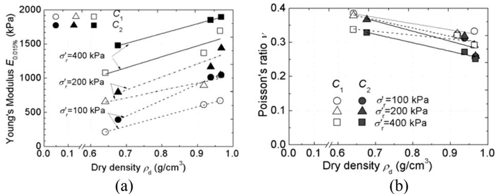
Figure 8: Variations of strength parameters with initial dry density and confining pressure: (a) Young's modulus and (b) Poisson's ratio
