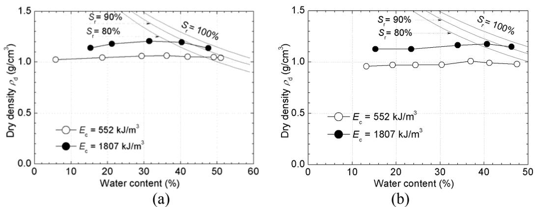
Figure 3: Dry density versus water content: a)  $C_1$  and (b)  $C_2$
