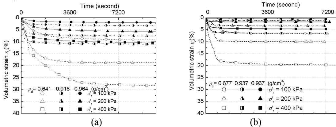
Figure 5: Volumetric strain during the consolidation: (a)  $C_1$ , (b)  $C_2$
