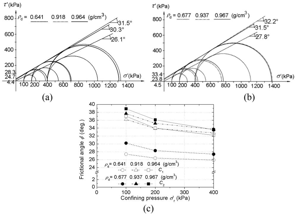
Figure 7: (a) Mohr envelope lines of  $C_1$ , (b) Mohr envelope lines of  $C_2$  and (c) The variation of frictional angle ( $\phi$ ) to the confining pressure.
