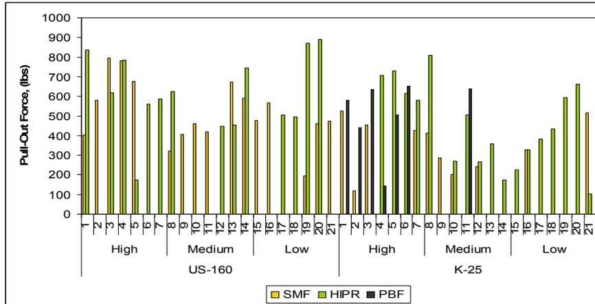
Figure 5: Pull off strength at different residual tack coat application rates on US-160 and K-25
