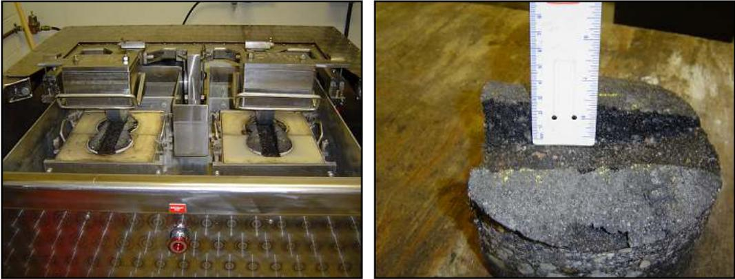
Figure 2: Experimental set-up and failure surface on field cores
