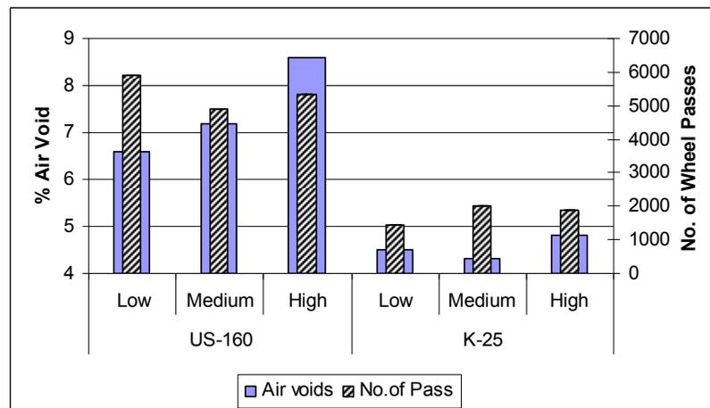
Figure 4: Rutting performances of field cores on US-160 and K-25
