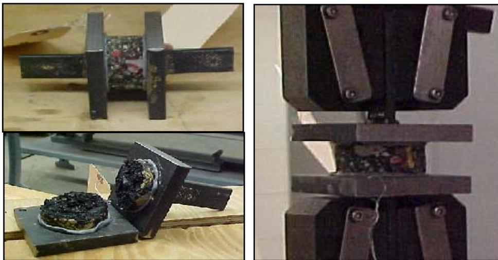
Figure 3: Pull-off strength test of tack coat material
