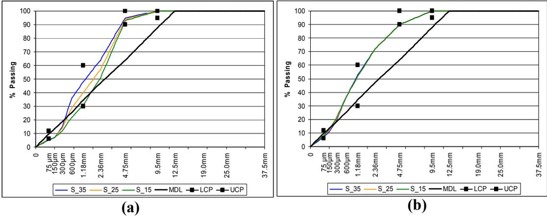
Figure 1: 0.45 power charts for 4.75-mm NMAS laboratory mixture (a) US-160 and (b) K-25
