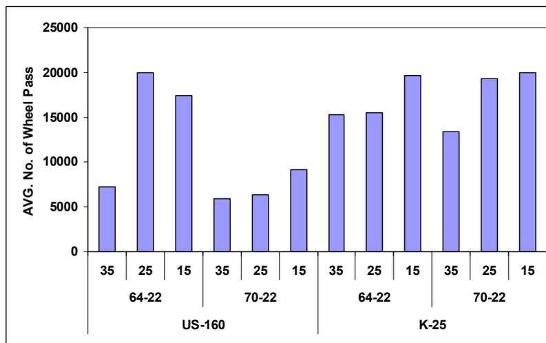
Figure 6: Rutting performances of 4.75-mm NMAS laboratory mixes
