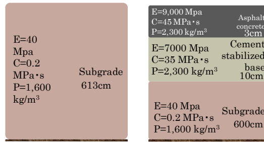
Figure 1: Semi-infinite model (left) and three layer pavement model (right)
